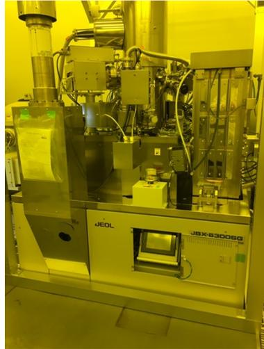
**Figure 3.2:** *EB lithography machine (model: JBX-6300FS) from JEOL company, which can easily write patterns down to 8 nm or less (actual result: 5 nm) by the employment of an electron optical system that automatically adjusts a 2.1 nm-diameter electron beam at a 100 kV accelerating voltage.*
