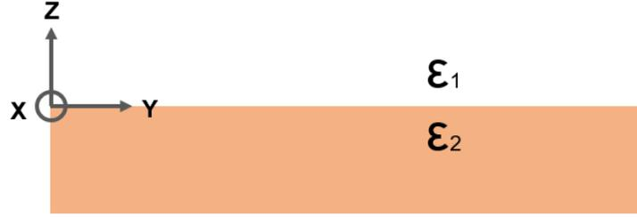
**Figure 2.2:** Schematic of a system consisting of two media, which are separated by a plane interface.  $\epsilon_1$  and  $\epsilon_2$  refer to dielectric functions in medium 1 and medium 2, respectively.
