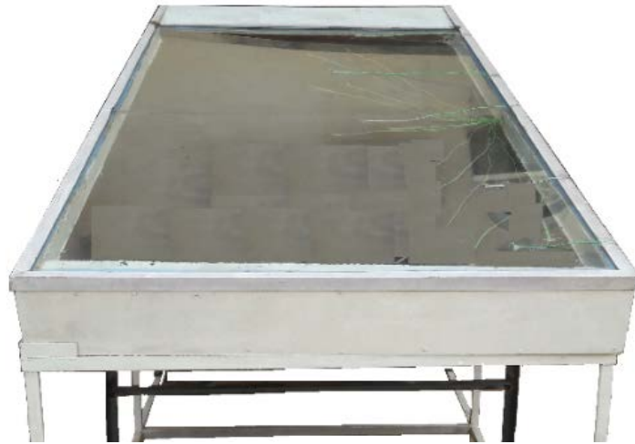
Figure 1. Picture of the double air pass solar thermal collector.
