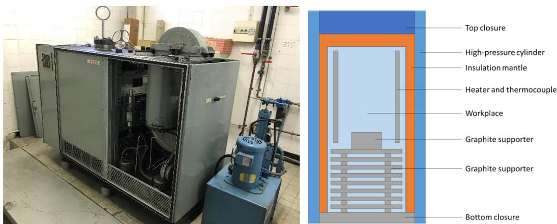
**Figure 2.7** (Left) ASEA QIH3 HIP system; (Right) Schematic drawing of HIP heating chamber.
