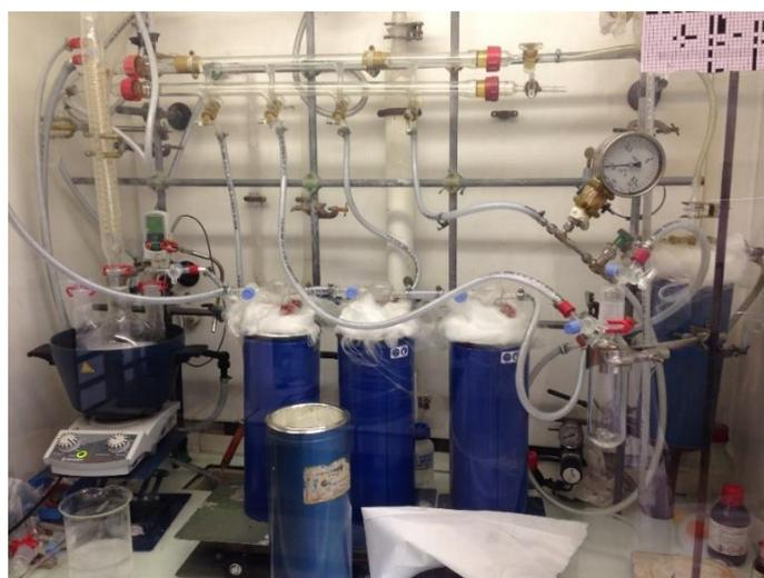
**Figure 2.1** Experimental set-up for borazine synthesis. On the left: flask where reaction occurs. In the middle: three collectors immersed in liquid nitrogen. On the right: a piezometer connected with a vacuum pump.
