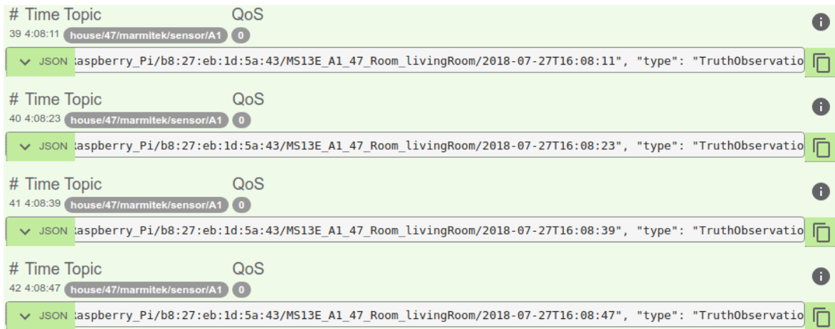
Fig. 4.13 MQTT-Communicated Sensor Event Example
