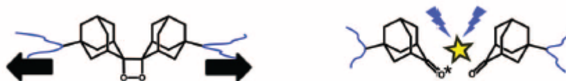
Figure 16: schematic representation of the breakage of the dioxetane crosslinker resulting in a photon emission [25].
