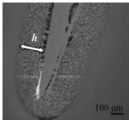
Figure 6: High-low image of the crack tip after tearing, captured using a colour 3D violet laser scanning microscope[29]
