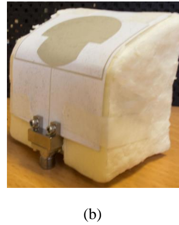
Figure 4.17. Study of bending effects of “Mushroom-shaped with two arms” antenna: (a) CST simulation structure with illustration of tilted angle \varepsilon_\theta and the bending position h ; (b) Experimental realization.
