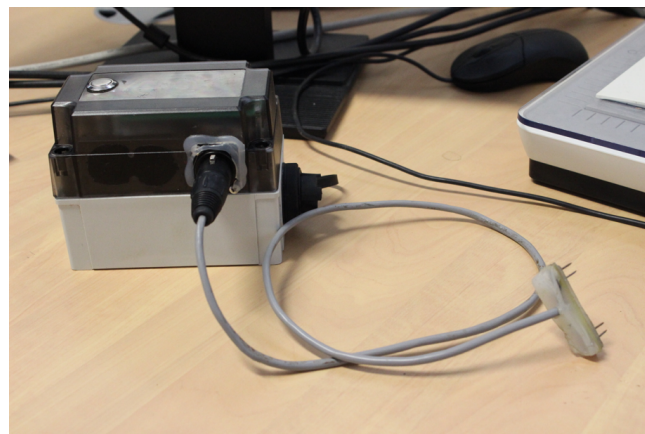
FIGURE 3.4: AD5933 Hand-held bioimpedance measurement system
