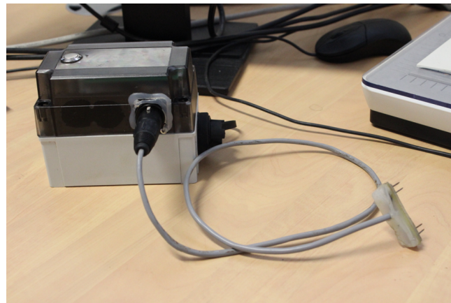
FIGURE 3.4: AD5933 Hand-held bioimpedance measurement system
