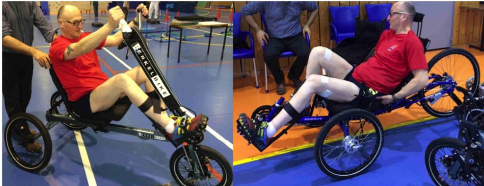
Figure 39. Comparison of the two recumbent trike used during the initial training program (on the left, the Berkelbike Pro) and for the final training program and at the competition (on the right, the FreeWheels trike).
