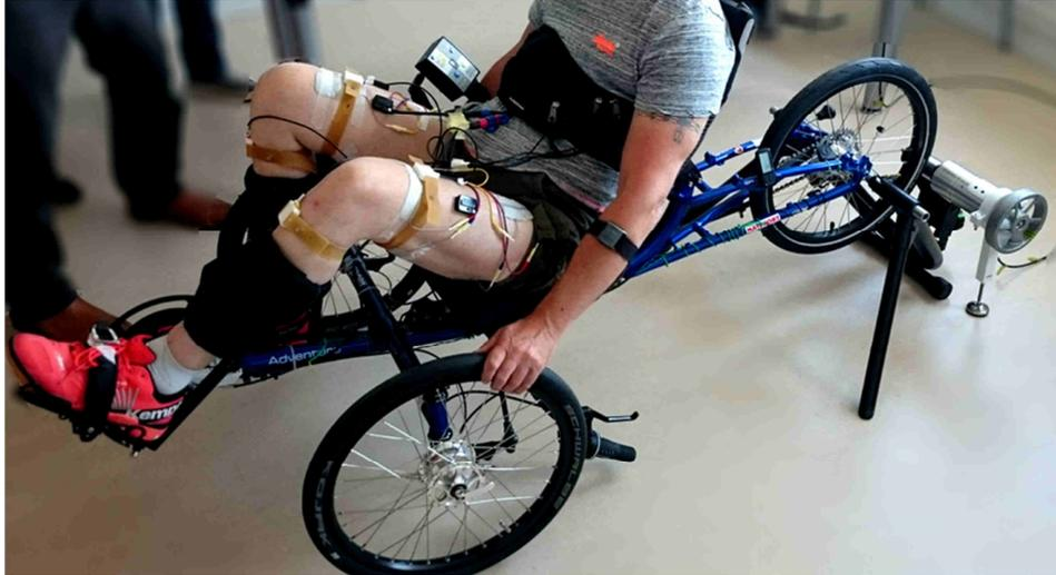
Figure 46. The SCI participant is equipped with IMUs, surface electrodes, EMG sensors and a heart rate arm band monitor. The power produced is recorded at the rear wheel via a rotating torquemeter.
