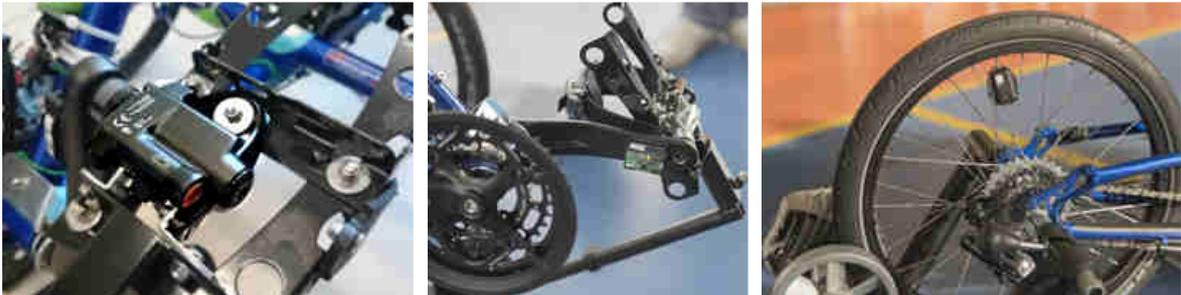
Figure 45. Cycling instrumentation: power pedals and IMUs were mounted on the trike for monitoring the pilot's performances.
