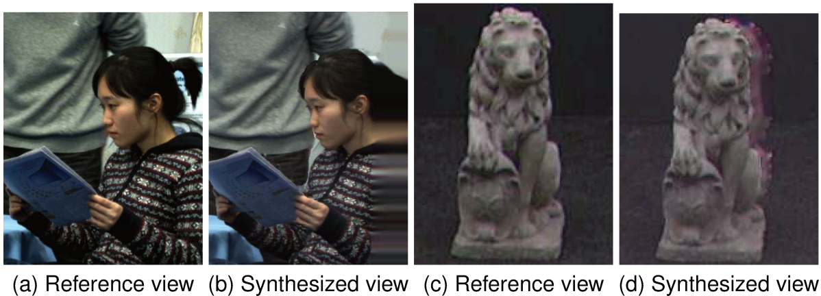
Figure 1.8: Synthesis distortions caused by imperfect image inpainting method. (a) and (b) stretching; (c) and (d) blurry regions. The “girl’s ” hair and clothes in image (b); and the right border of the sculpture in (d).
