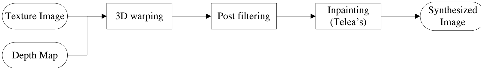
Figure 4.6: Block diagram of VSRS
