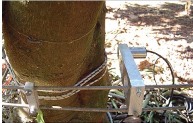
Figure 10 – Photograph of LVDT sensor device for measuring diameter fluctuations in trunks of citrus tree [Ortuno, 2010]
