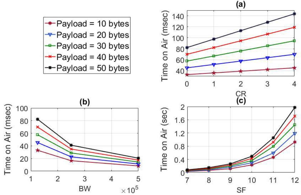
Figure 4.3:  $LoRa^{TM}$  packet time on air (a)  $SF = 7$  and  $BW = 125$  kHz (b)  $SF = 7$  and  $CR = 0$  (c)  $CR = 0$  and  $BW = 125$  kHz
