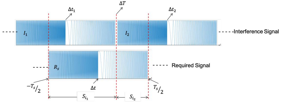
Figure 4.9: Interfering LoRa symbols at receiver.
