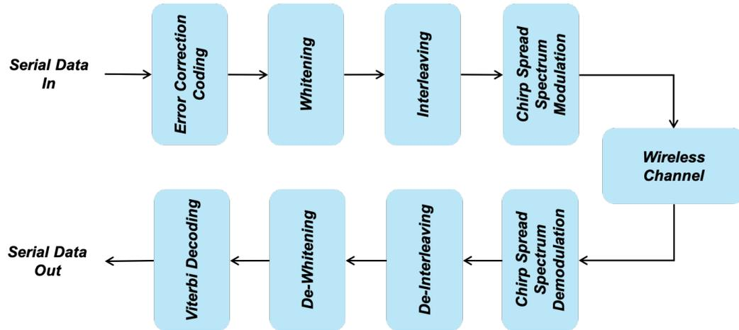
Figure 4.5: *LoRa*<sup>TM</sup> PHY layer architectureTableau 4.1: Error detection and correction capabilities of *LoRa*<sup>TM</sup>.
