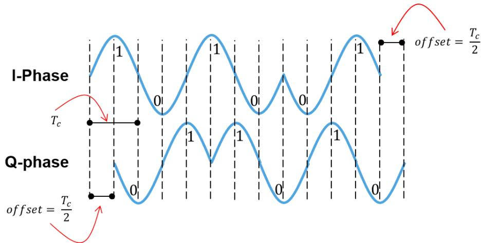
Figure 3.17: O-QPSK pulse shaping with half sinusoid waveform.
