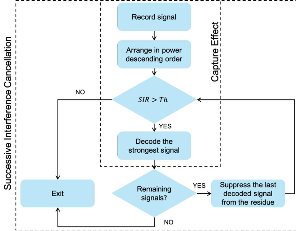
Figure 4.16: Block diagram for CE and SIC
