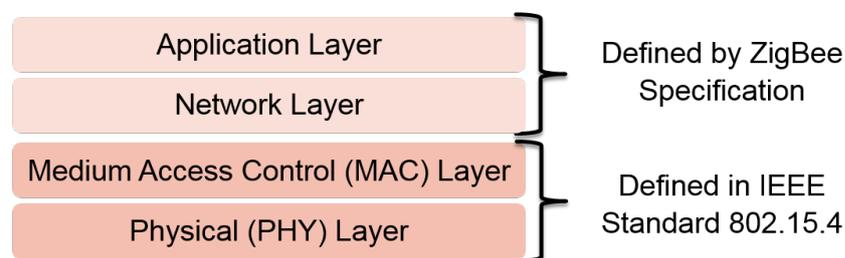
Figure 3.11: IEEE 802.15.4 and ZigBee protocol stack architecture
