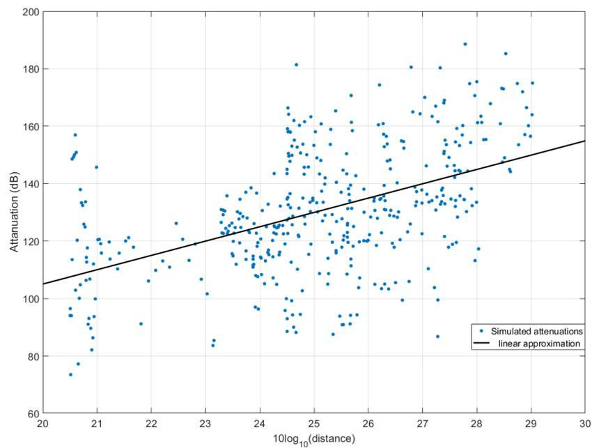
Figure 3.26: Attenuation as function of distance.
