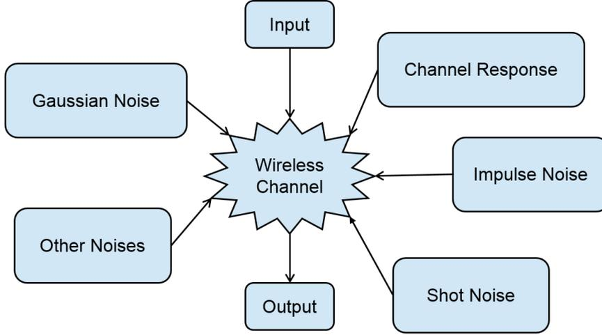
Figure 1.9: Characterization of noise in wireless channel.
