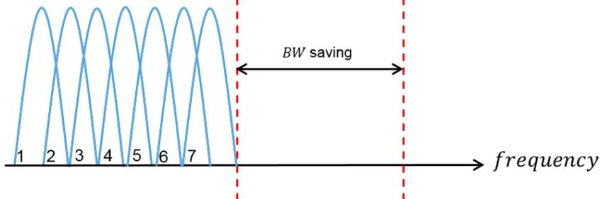
Figure 3.4: orthogonal signals concept
