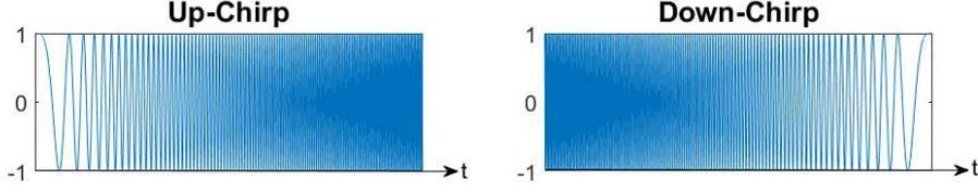
Figure 4.6: Up-chirp and down-chirp signal.
