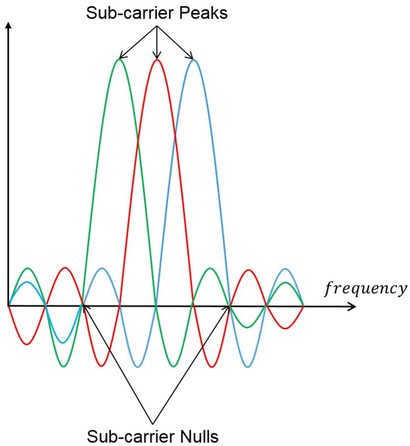
Figure 3.6: Orthogonal subcarriers in multicarrier systems (OFDM)
