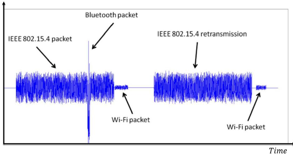
Figure 2.5: Zigbee, Wi-Fi and Bluetooth packet interference.
