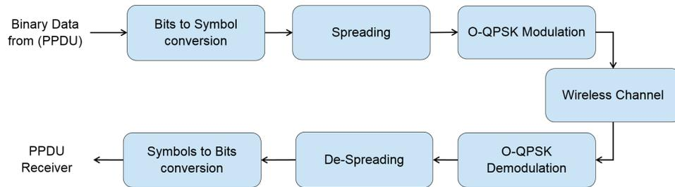
Figure 3.15: Functional block diagram of IEEE 802.15.4 transceiver.
