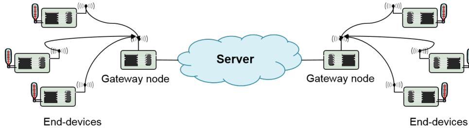
Figure 4.1: *LoRaWAN<sup>TM</sup>* network structure.
