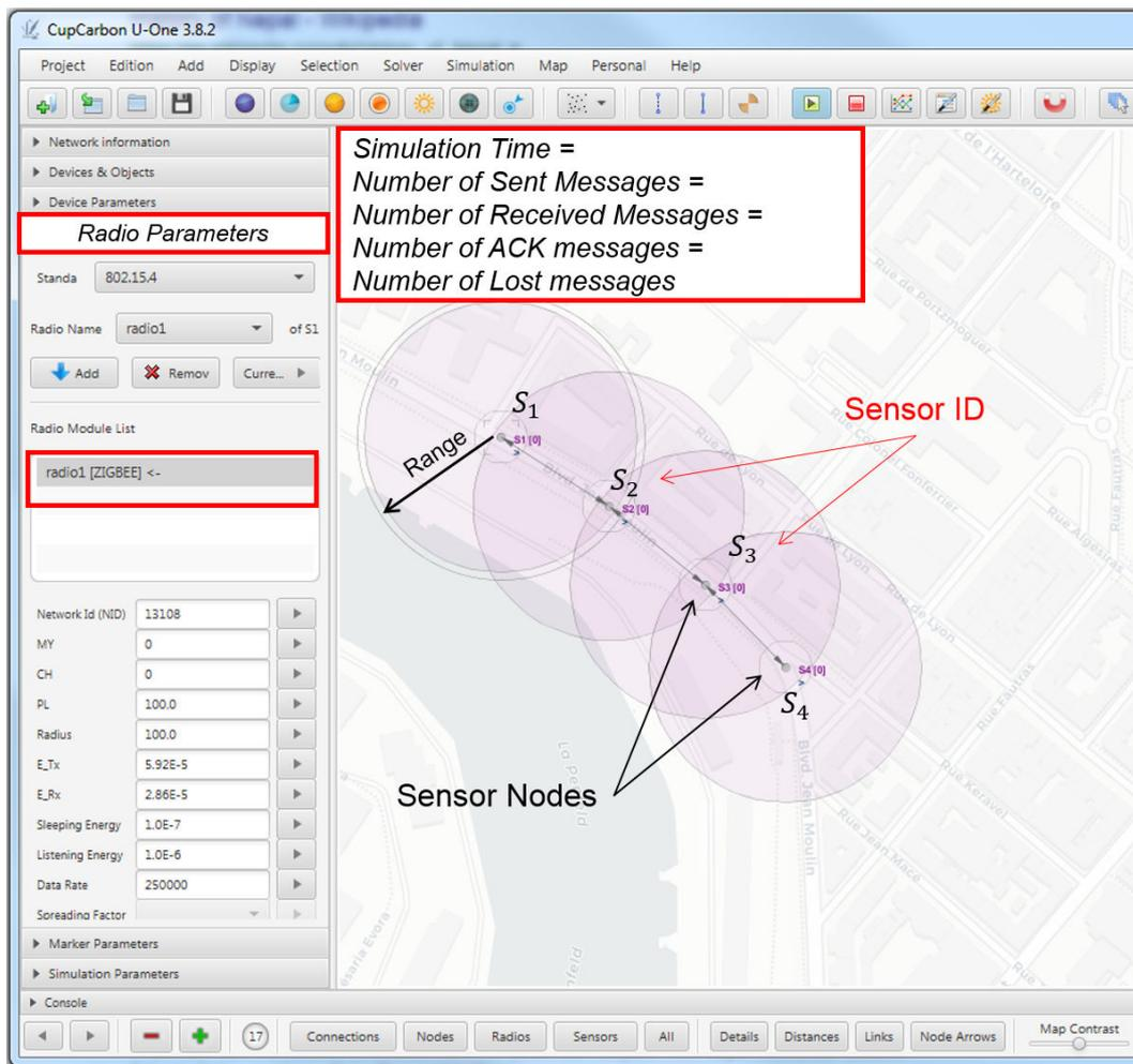
Figure 3.36: Radio parameter settings in CupCarbon.
