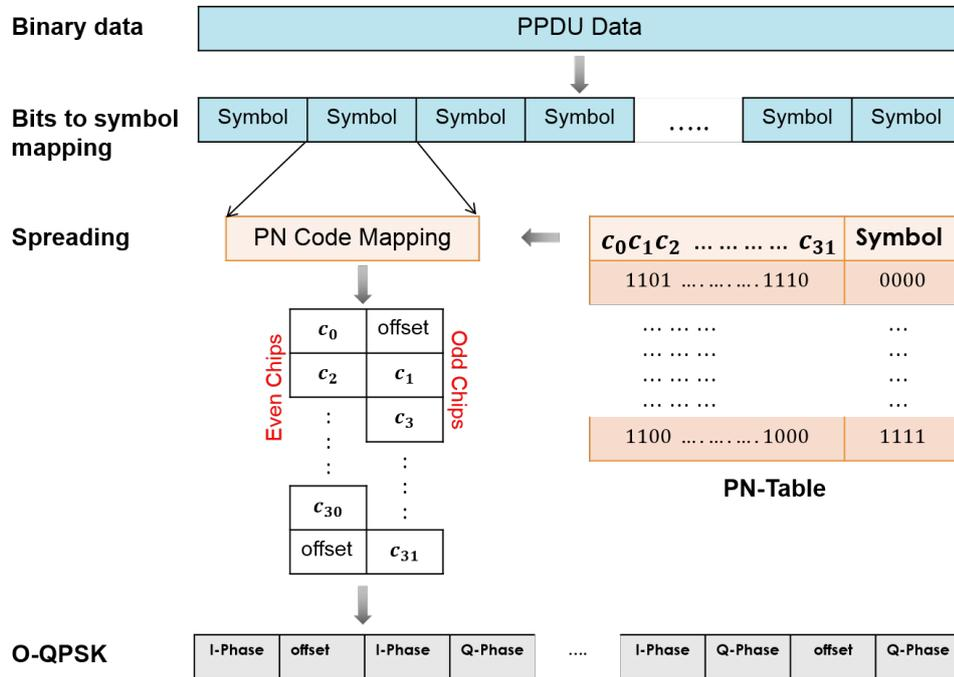
Figure 3.16: ZigBee transmitter operations.
