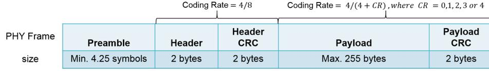
Figure 4.2: *LoRa<sup>TM</sup>* PHY frame format
