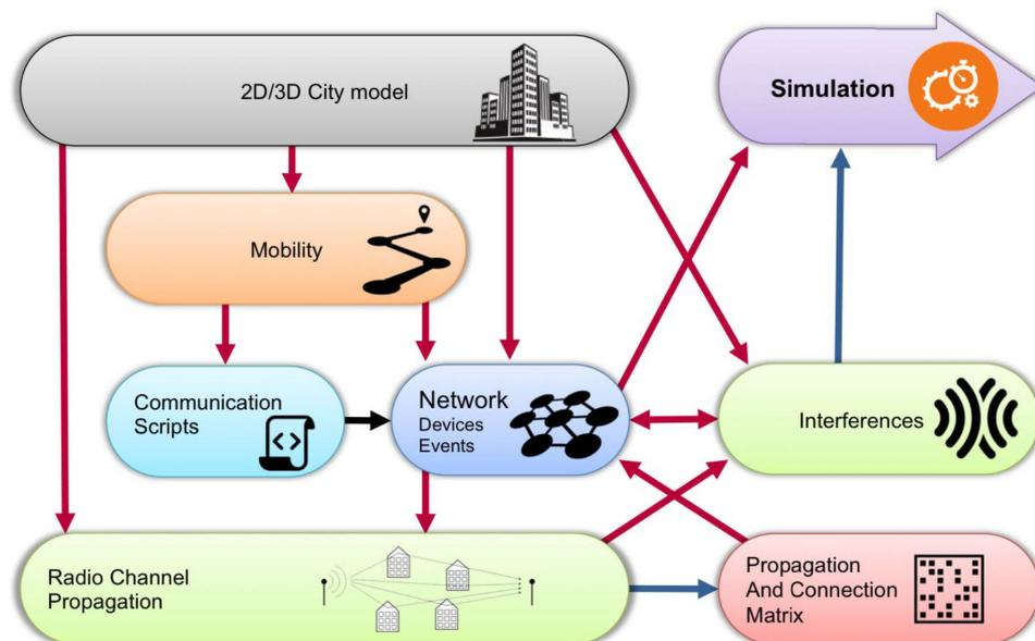
Figure 2.7: Main components of the CupCarbon architecture.
