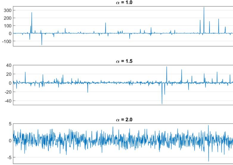
Figure 1.12: Distribution of noise impulses using different values of  $\alpha$ .
