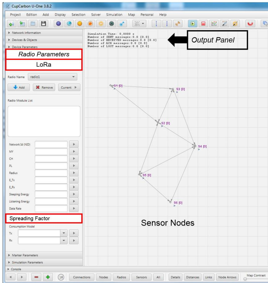
Figure 4.20: Radio parameter settings for LoRa in CupCarbon.
