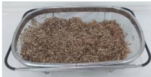
Figure V-3. Sample of hemp shiv aged during two years in A_{Ext} conditions
