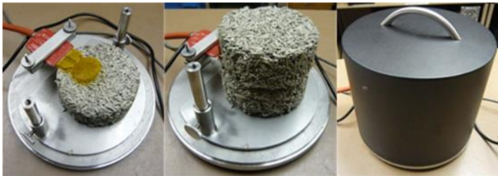
Figure IV-5. Hot Disk system with specimens of hemp concretes
