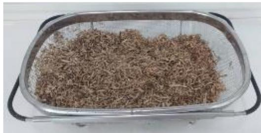
Figure V-3. Sample of hemp shiv aged during two years in  $A_{Ext}$  conditions
