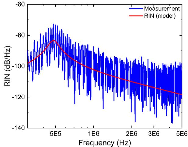
Figure 2-24: Relative intensity noise measurement and fit.
