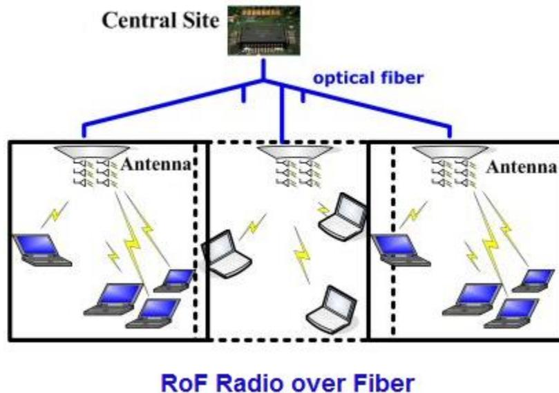
Figure 1-2. Example of a radio over fiber architecture [7].
