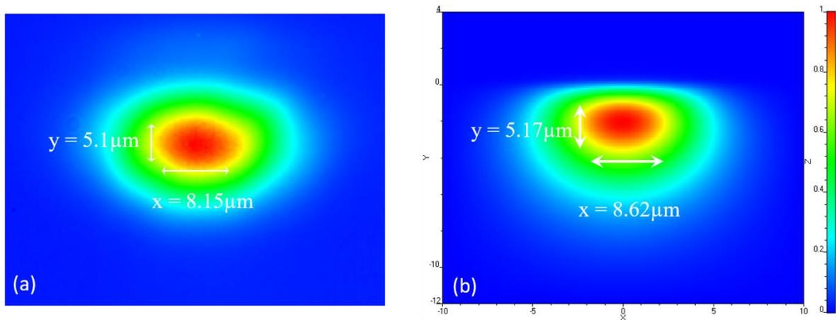
Figure 2-6. Mode profile for a  $7\ \mu\text{m}$  wide waveguide ion-exchanged at  $T = 320\ ^\circ\text{C}$  for a duration  $t = 7\ \text{min}$  at  $\lambda_s = 1550\ \text{nm}$ : a) Measurement and b) Simulation.
