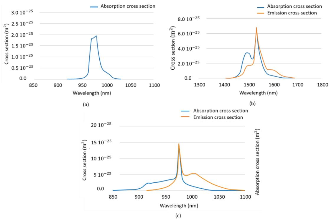
Figure 2-2. (a) absorption cross section around  $\lambda_{\text{p}}$ , (b) absorption and emission cross sections around  $\lambda_{\text{s}}$  for the  $\text{Er}^{3+}$  ions and (c) absorption and emission cross sections around  $\lambda_{\text{p}}$  for  $\text{Yb}^{3+}$  ions in IOG1 glass Source: data sheet of the manufacturer [45].
