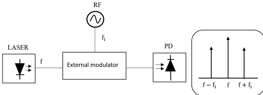
Figure 1-8 Frequency generation using an external modulator.
