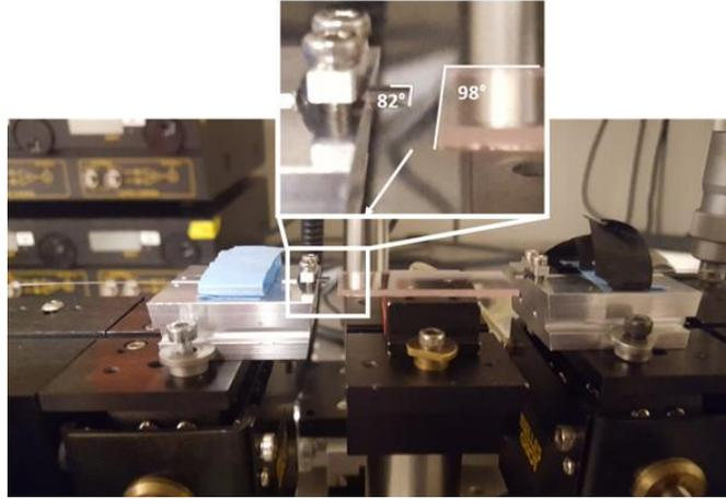
Figure 2-15 Photography of the optical bench on which a 98° polished sample and a 82° ferrule are maintained.
