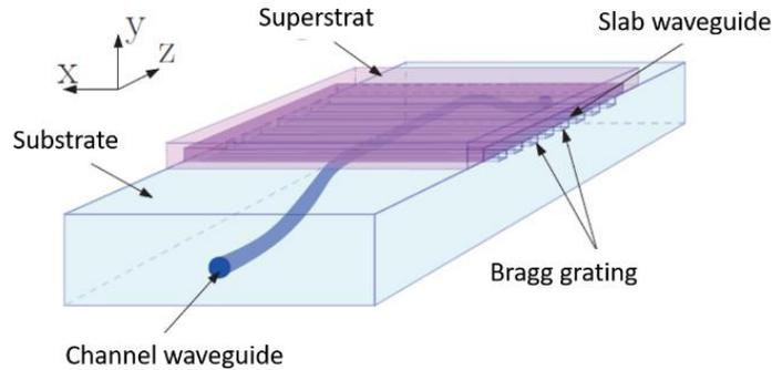
Figure 1-17 Three-dimensional hybrid DFB laser on glass substrate [42].
