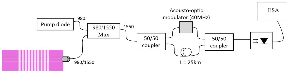
Figure 2-21 Self-heterodyning setup used for linewidth measurement.
