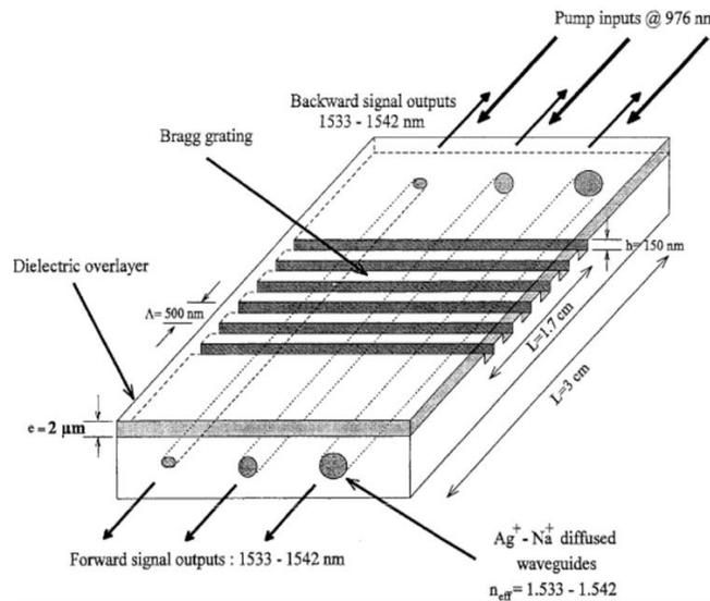
Figure 1-16 Glass integrated optics laser matrix [44]
