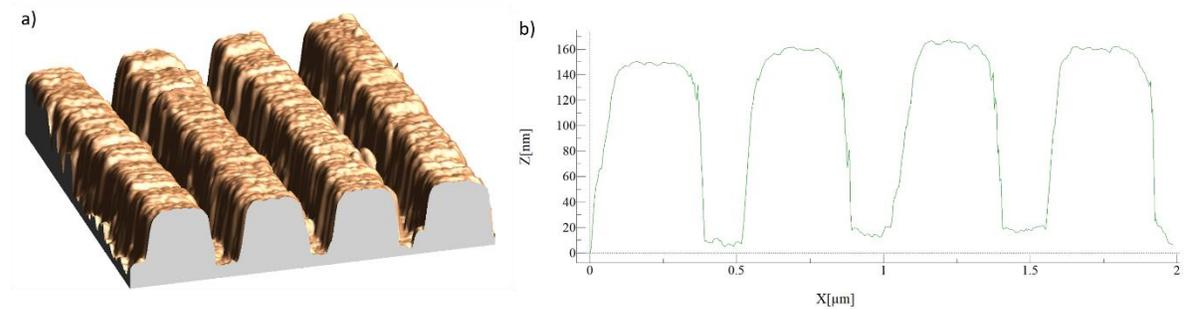
Figure 2-14 Bragg grating a) AFM image, b) profile.
