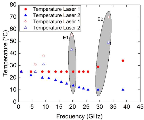
Figure 3-9 Generated frequencies for different lasers temperatures setting couples.
