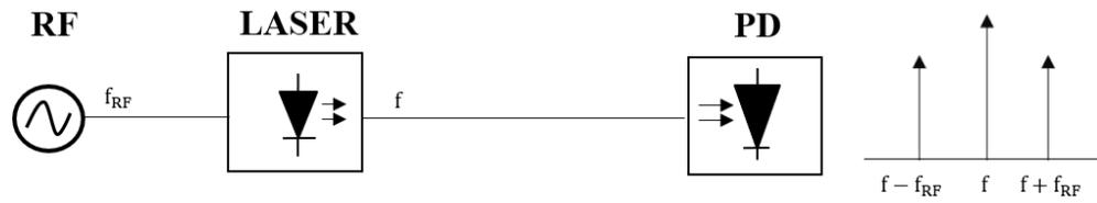
Figure 1-7. Frequency generation using direct modulation technique.
