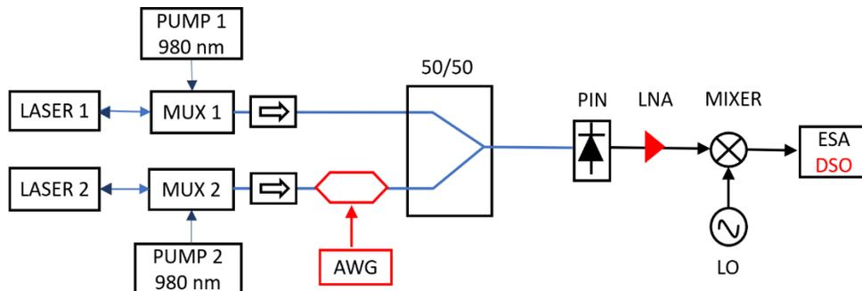
Figure 3-19 Experimental setup for data transmission measurements.
