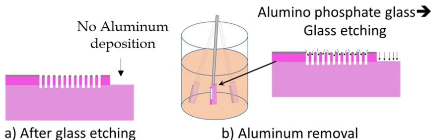
Figure 2-13 Aluminum removal process
