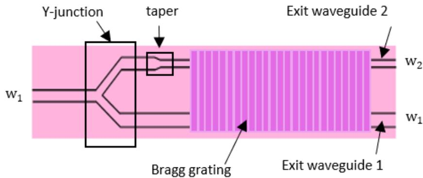
Figure 4-6 Co-integrated lasers with a Y-junction.
