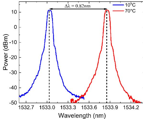
Figure 2-19 Laser emission spectra at 10 °C and 70 °C.
