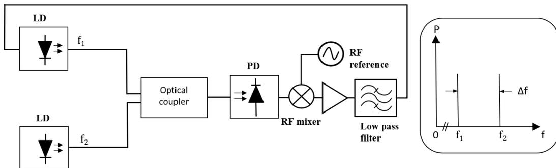
Figure 1-10 Optical phase lock loop setup.
