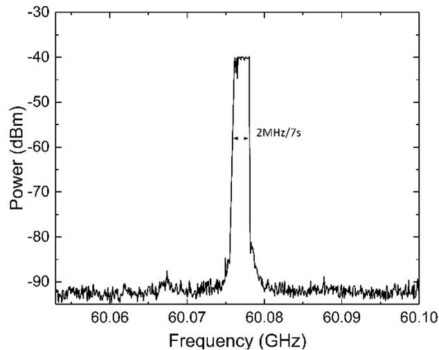
Figure 3-16. Measured frequency deviation for configuration C at 60 GHz.
