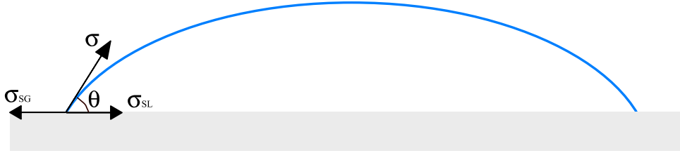
FIGURE 1.2: Two-dimensional representation of a droplet on substrate describing interfacial tensions.
