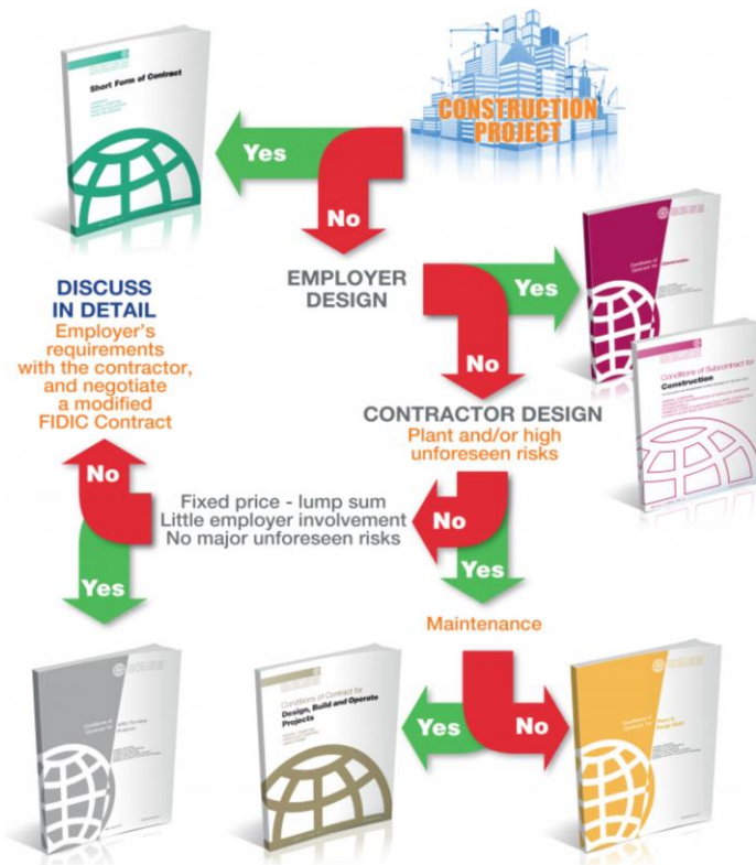
Figure 25 : FIDIC contracts and how to use them (FIDIC, 2018). FIDIC contracts are example of the different types of contracts existing for construction systems abroad.
