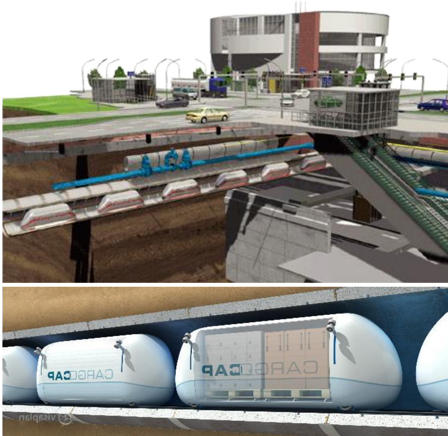
Figure 214 : Cargocap example of an underground logistic system to transport freight (CargoCap, 2007).
