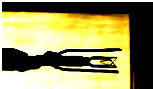
Figure 3.11 - Air pockets behind the two-component hot-film probes
