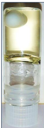
Figure 4.15 Inverted vial test for one of the synthesized hydrogels.
