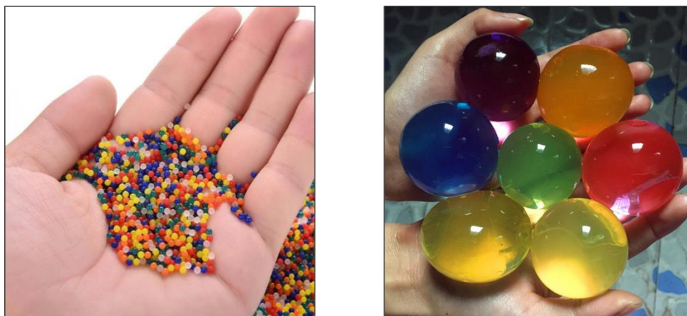
Figure 3.1 Example of polyacrylates hydrogels swelling behavior.
