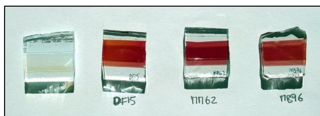
Figure 2.20 TiO 2 films on glass sheets, from left to right: untreated; sensitized with DF15 ; sensitized with MM62 ; sensitized with MB96 .
