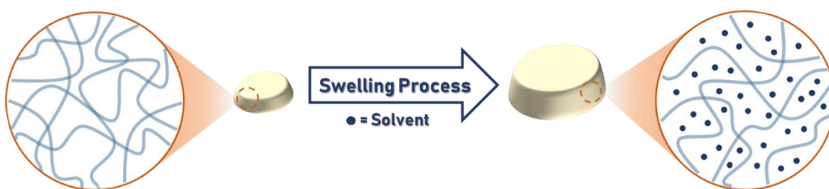
Figure 3.14 Schematic representation of the swelling process.
