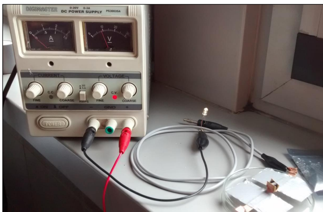
Figure 4.25 Demonstration of the conductivity of the conductive hydrogels developed by powering a small LED.
