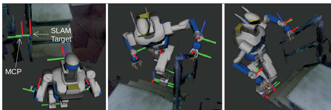
Fig. 3.12 Combined view of the stairs climbing experiment. The left figure shows the gripper's grasping pose (leftmost frame) that would have been tasked by the MCP without registration, and the corrected registered grasping frame onto the handrail. The others show HRP-2Kai climbing the first step.
