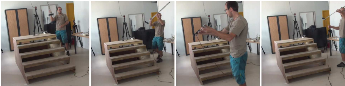
Fig. 2.10 Images from the calibration sequence, camera-ruler calibration is moved by hand around the staircase, camera motion is tracked with SLAM while the ruler motion is tracked with the VICON MOCAP system to provide input data for Hand-Eye calibration
