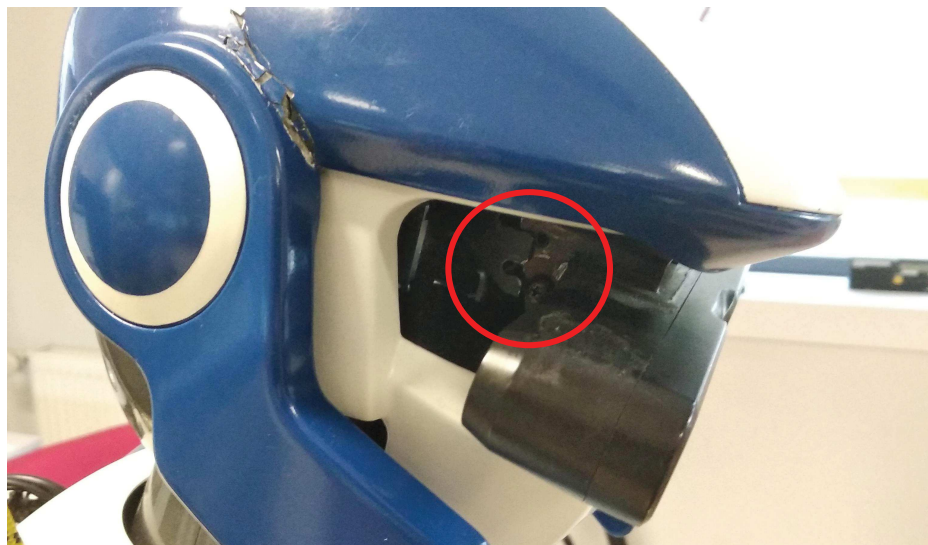
Fig. 2.1 During a stair-climbing experiment, HRP-4 fell on its supporting rope, which damaged the mechanism holding the Asus Xtion in place. This illustrates the importance of having an autonomous online calibration method for robust operation in real environments.
