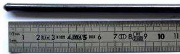
Figure 3.5 – As-grown single-crystal of \text{Nd}_2\text{NiO}_{4+d} , with d=0.22-0.25 , obtain through TSFZ growth on the NEC SC3-MDH11020 mirror furnace. The single-crystal is homogeneous and one-time twinned. Figure from reference [1].
