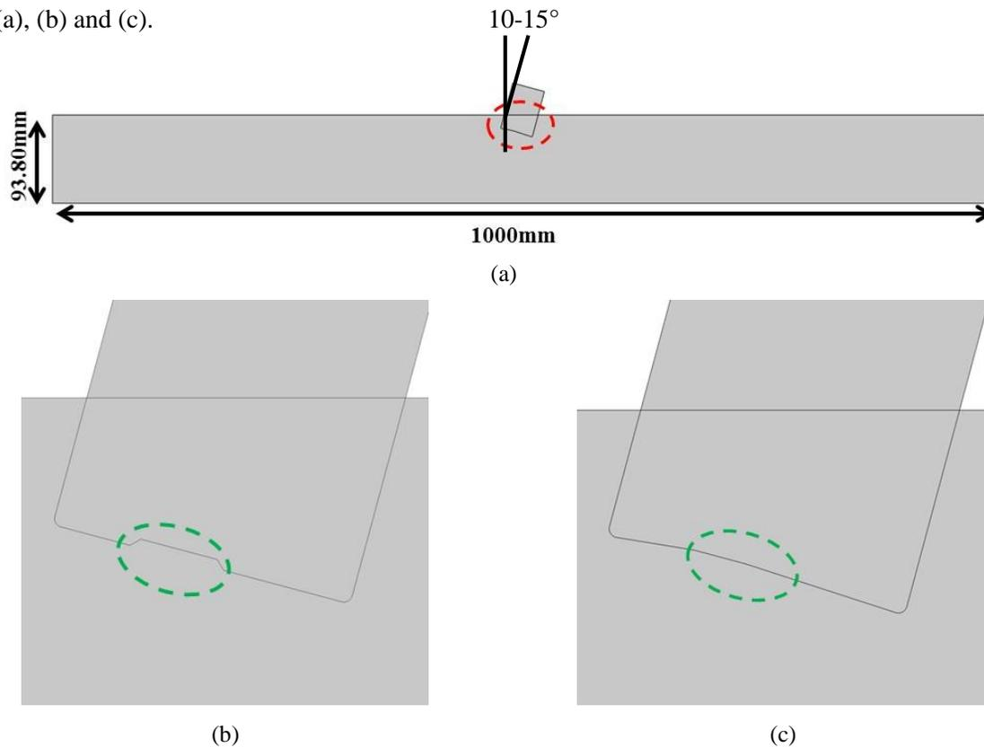
Figure 4-31: (a) The picture of the round-edged sensor node tilted at  $15^\circ$  with respect to the normal and inserted into a water pipe, (b) the sensor node head chamfered with a 0.5 mm radius and (c) 1 mm radius.
