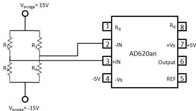
Figure 2-9: Schematic diagram of the data reading circuit. Here, the Wheatstone bridge consists of four resistors  $R_1$ ,  $R_2$ ,  $R_3$  and  $R_4$  represent the four piezoresistors of the pressure sensor.
