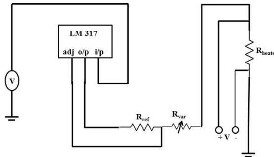
Figure 4-13: Schematic of the constant current circuit source.
