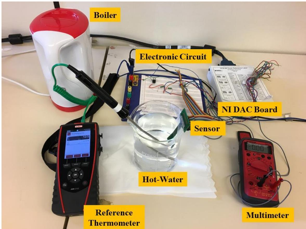
Figure 3-3: Experimental setup for the temperature sensor Calibration.
