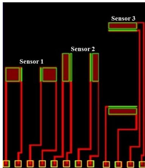
Figure 2-13: Different versions of the conductivity sensor
