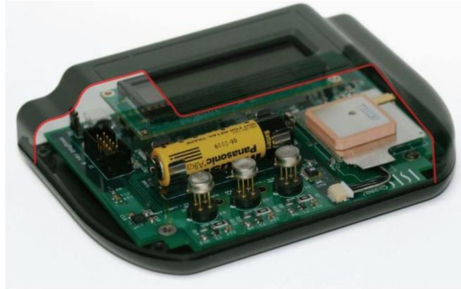
Figure 1-2: The Mobile sensor node
