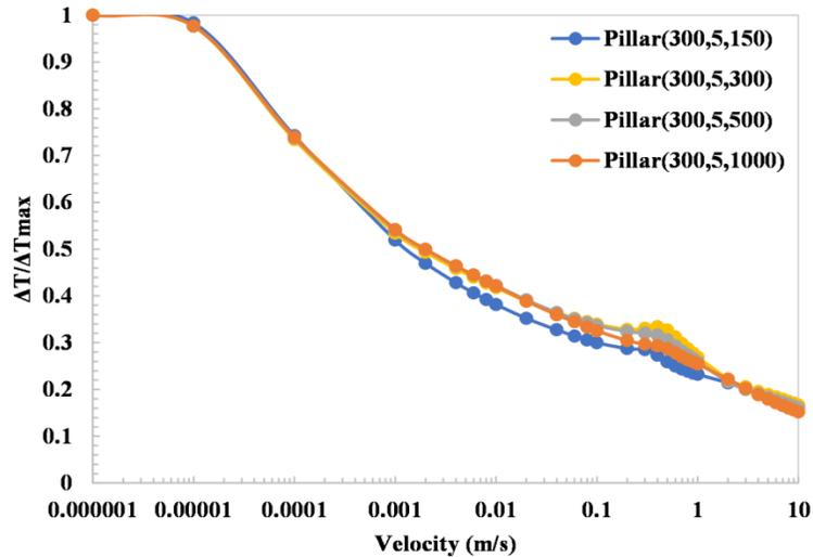
Figure 4-27: Pillar structure flow-rate sensor response as a function of fluid velocity for different cavity depths. Numbers between parentheses in the legend indicate the pillar height (equal to the cavity depth) and width then the cavity width, respectively.
