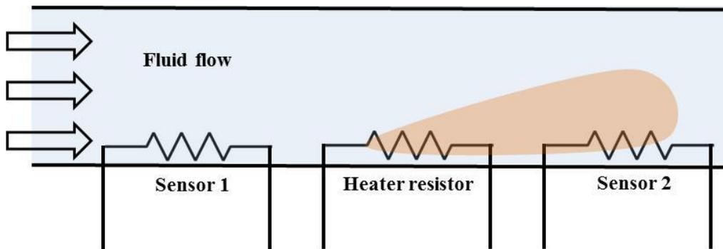
Figure 4-9: Schematic representation of calorimetric operation mode of a thermal flow-rate sensor <sup>82</sup>
