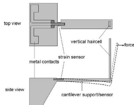
Figure 4-7: Schematic representation of single hair cell biomimetic flow-rate sensor <sup>111</sup>
