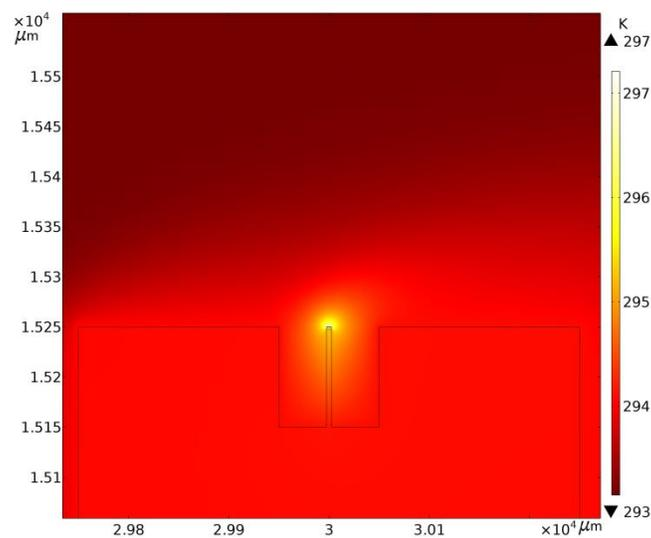
Figure 4-24: The temperature field of the pillar flow-rate sensor at 10 mW power supply at a velocity of 0.04 m/s. In this case, the cavity dimension is 150 x 100  $\mu\text{m}$  and the resistor width is 5  $\mu\text{m}$ .
