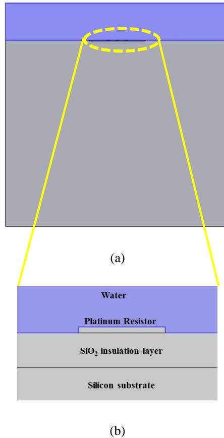
Figure 4-17: (a) Geometry of silicon substrate flow-rate sensor, and a (b) zoom picture of the platinum resistor and SiO<sub>2</sub> insulation layer
