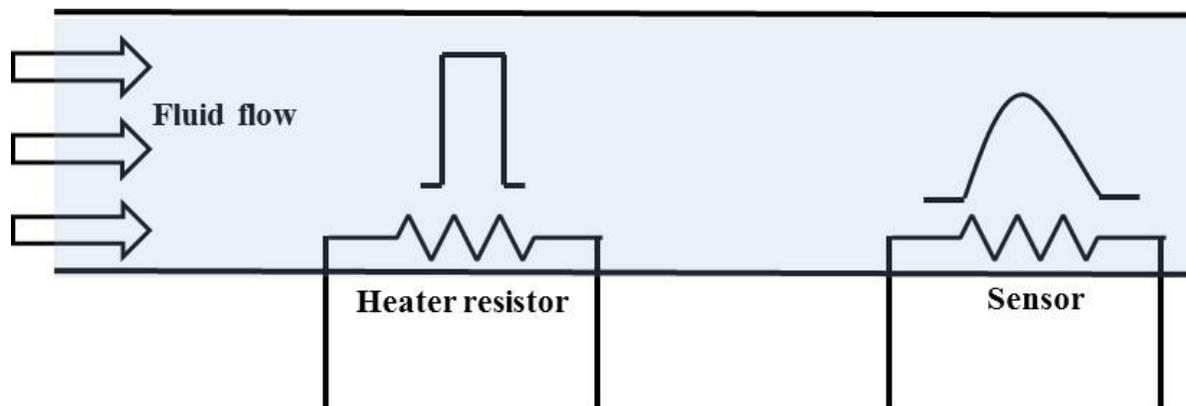
Figure 4-10: Schematic representation of Time-of-Flight operation principle of a thermal flow-rate sensor<sup>82</sup>
