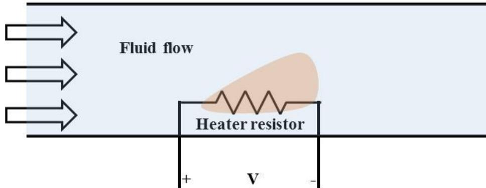
Figure 4-8: Schematic illustration of Hot-wire anemometer flow-rate sensor <sup>82</sup>
