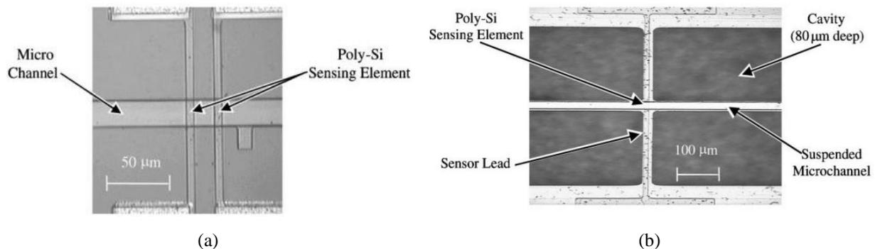
Figure 4-6: Fabricated flow-rate sensor (a) microchannel fabricated on the substrate and (b) a suspended microchannel<sup>110</sup>
