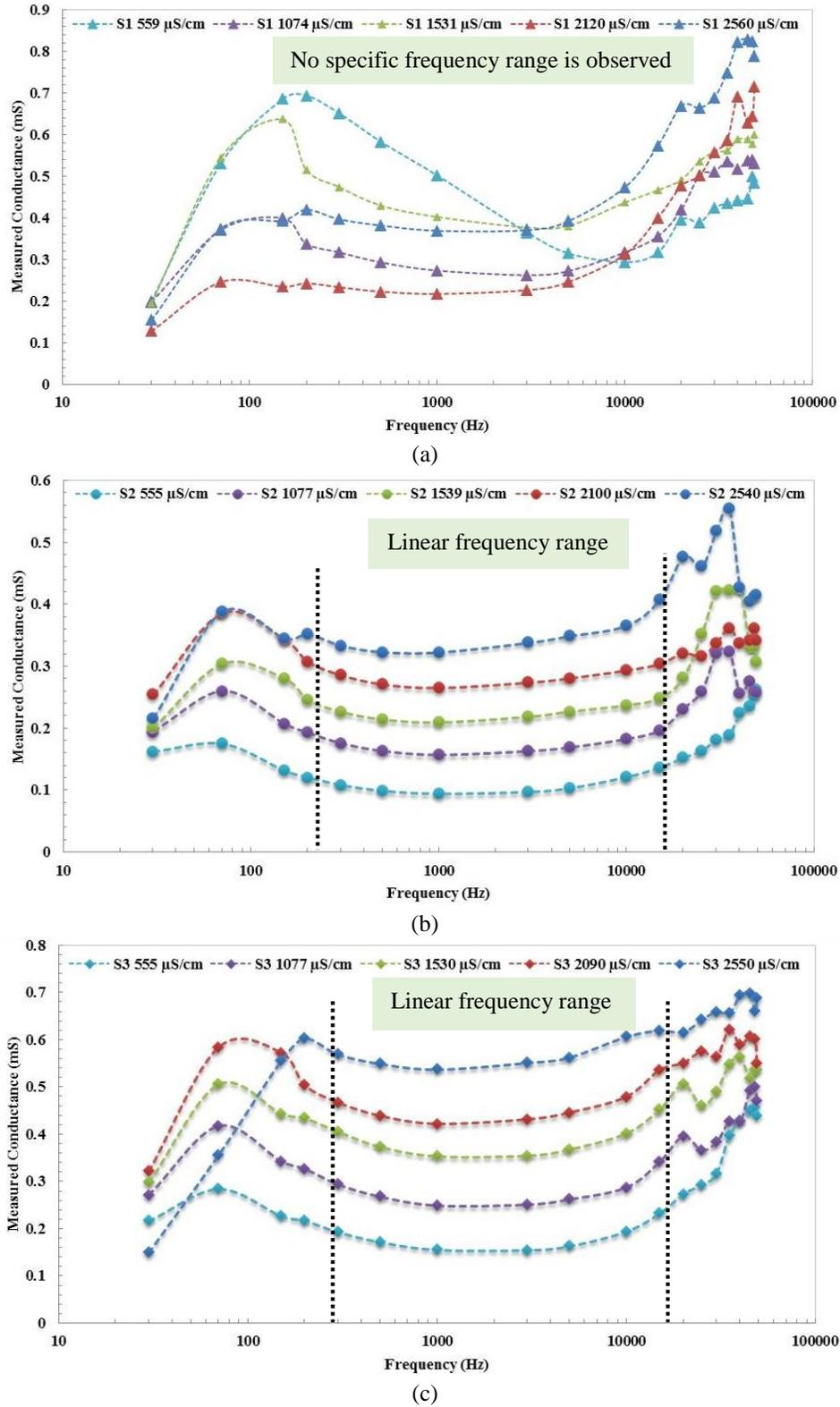
Figure 2-16: Responses of the three sensors in frequency sweep analysis (a) sensor 1, (b) sensor 2 and (c) sensor 3 under the frequency range  $\sim 500 \mu\text{S}/\text{cm}$  to  $\sim 2500 \mu\text{S}/\text{cm}$ .
