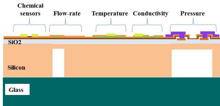
Figure 2-3: Cross-section view of the membrane-based flow-rate sensor
