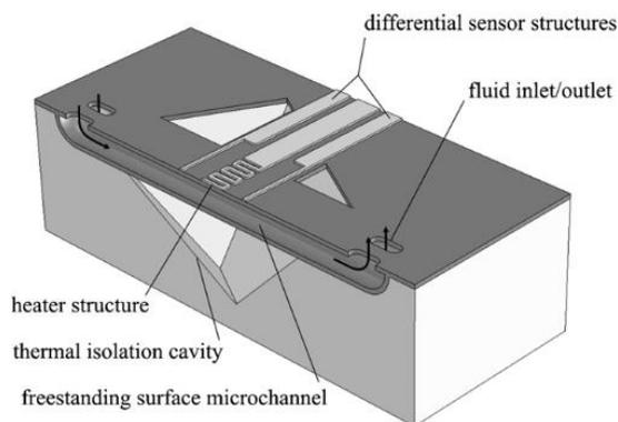
Figure 4-4: Cross-section view of a micro-machined flow-rate sensor<sup>109</sup>
