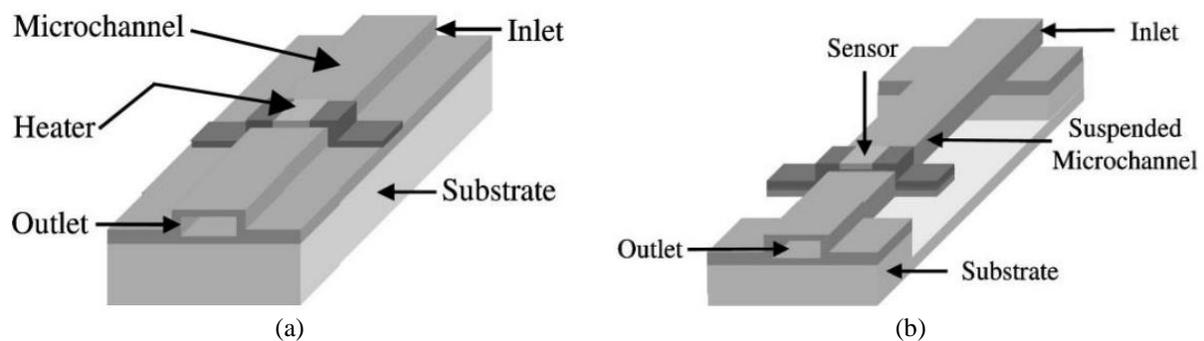
Figure 4-5: A microchannel flow-rate sensor, where the channel is fabricated on (a) the substrate and (b) in suspended configuration<sup>110</sup>
