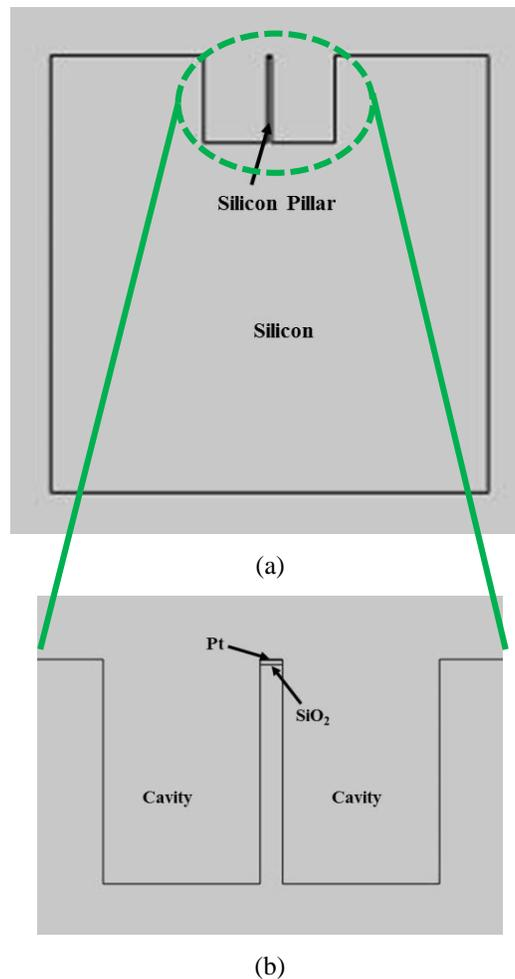
Figure 4-23: The pillar based flow-rate sensor geometric configuration.
