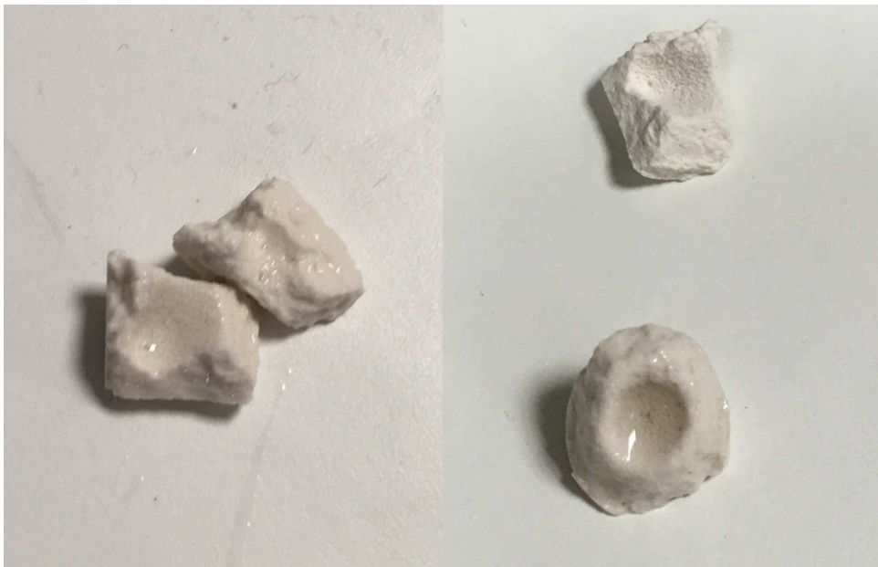
FIGURE 3.17: Remains of four stones after treatment of more that 7500 shocks at a 2 Hz PRF with a -5 kV input voltage pulse.
