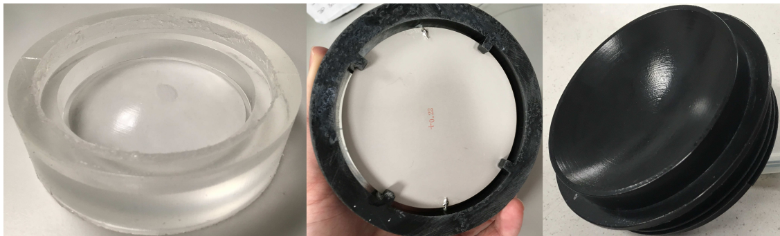
FIGURE 7.1: Left: RTV-141 silicone mold of the lens. Middle: 3D printed support for the ceramic with the ceramic glued in place. Right: the finished transducer.
