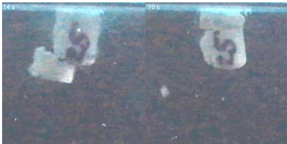
FIGURE 3.2: Example of an artificial stone that quickly broke in 3 parts after exposure to 180 kHz BWL. The white cross in the first photo represents the approximate position of the focus of the transducer. Acoustic propagation from bottom to top.
