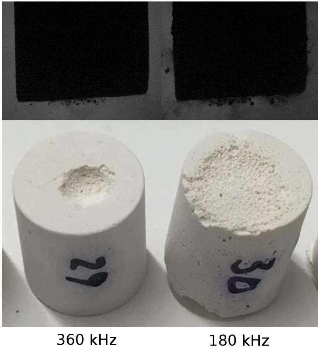
FIGURE 3.5: Top: High speed photographs of the stones during BWL with a shutter speed of 10 \mu s . Bottom: Photo of the proximal face of the stone after an exposure of 10 min of BWL.
