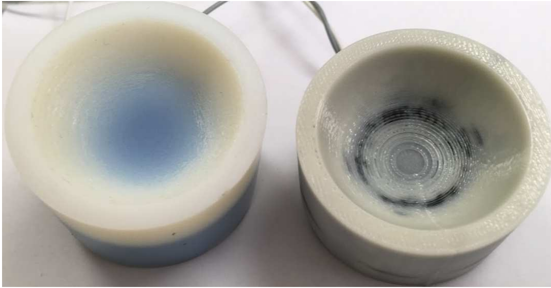
FIGURE 5.2: Left: single material lens, right: bi-layer lens.
