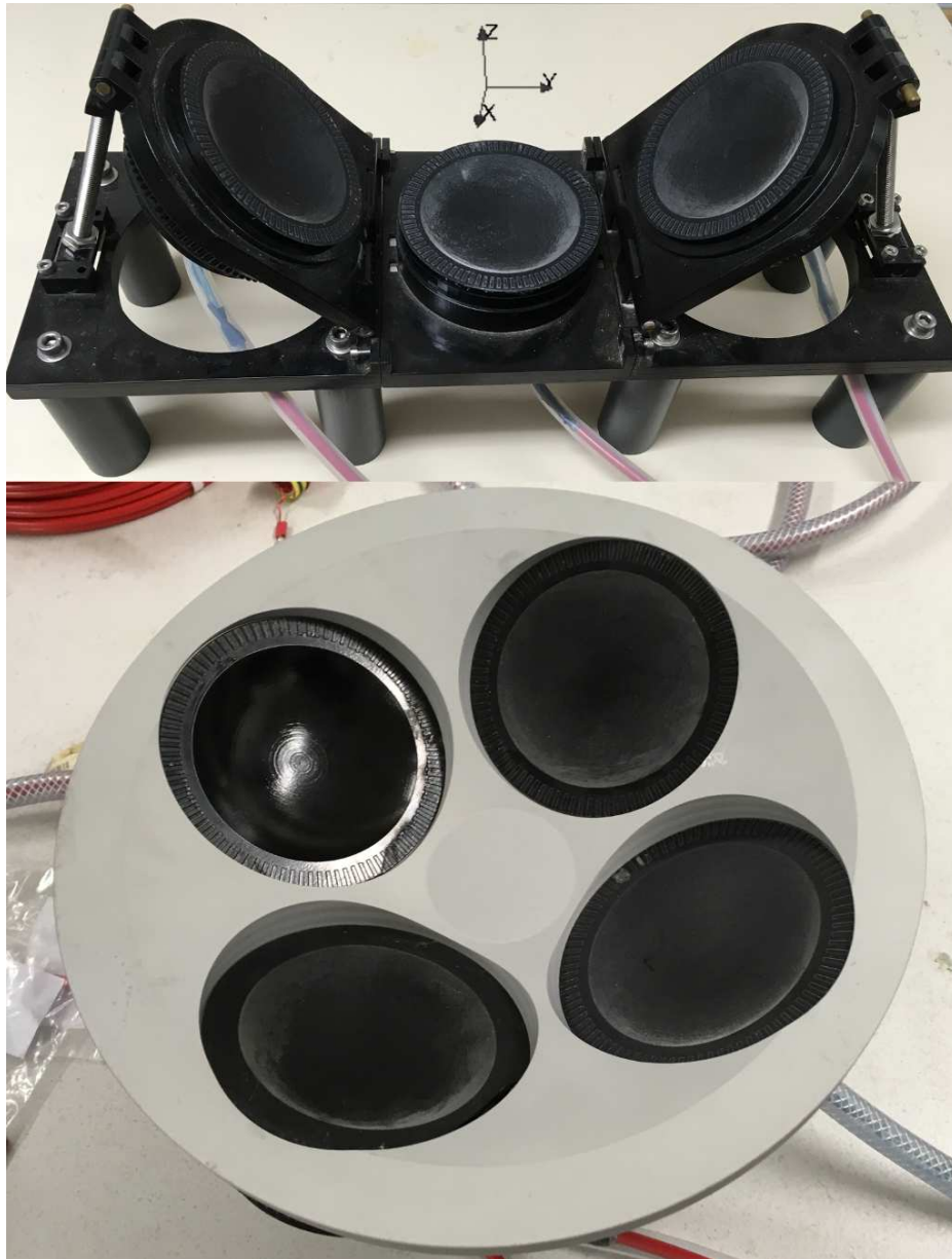
FIGURE 6.2: Top: Three transducers confocal setup. Bottom: Four transducers confocal setup.
