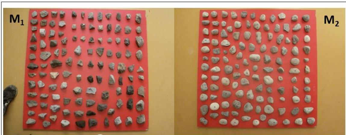
**Figure 2:** Example of pictures taken for roundness analysis for the angular pebbles sample M<sub>1</sub> (left) and the rounded pebbles sample M<sub>2</sub> (right).
