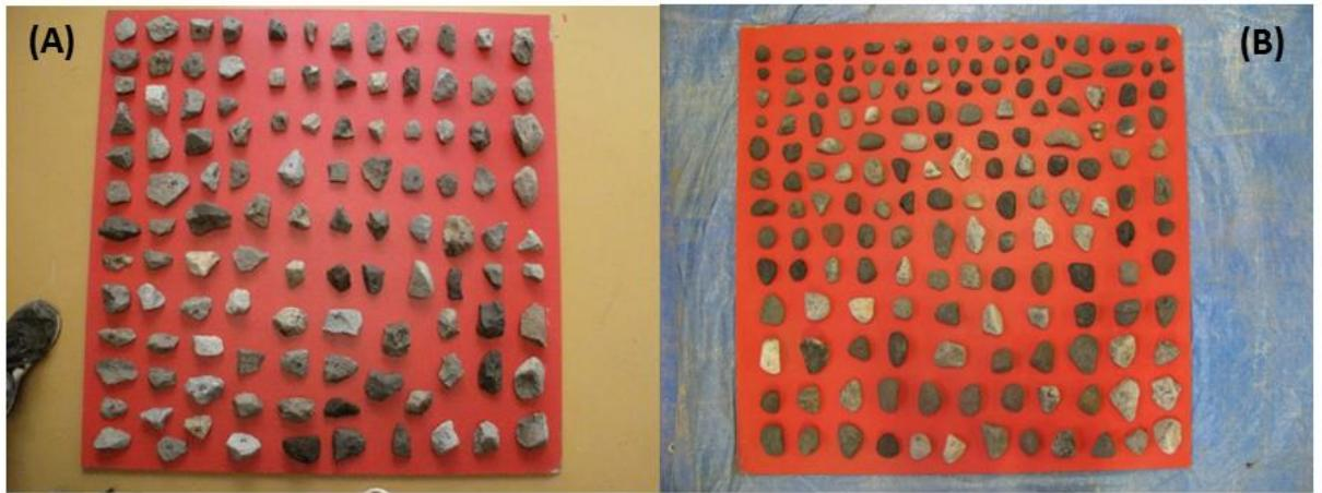
**Figure 9: Pictures taken for roundness analysis of the angular pebbles sample M<sub>1</sub> before (A) and after (B) abrasion runs.**
