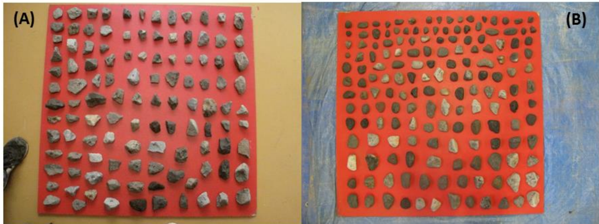
Figure 9: Pictures taken for roundness analysis of the angular pebbles sample M_1 before (A) and after (B) abrasion runs.
