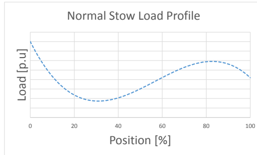
Fig. 6.8 Stow position dependent load profile shape
