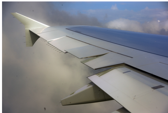
Fig. 5.7 Aileron control surface splitting on the Airbus A380 [2]
