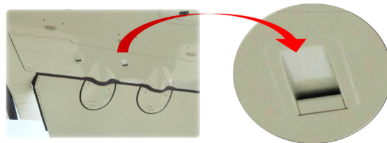
Fig. 5.4 Underwing scoops for actuator cooling (EHA of the Airbus A350 aileron) [152]
