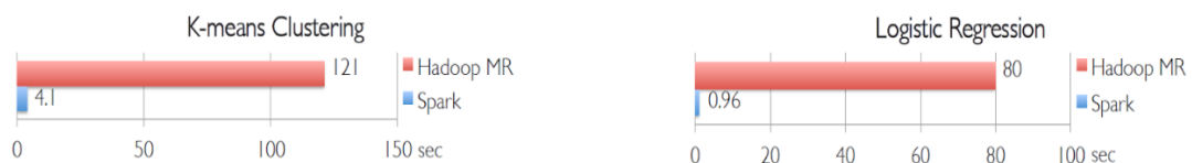
FIGURE 2.6: Running time of k -means and logistic regression in Hadoop and Spark [Zaharia et al., 2012a]
