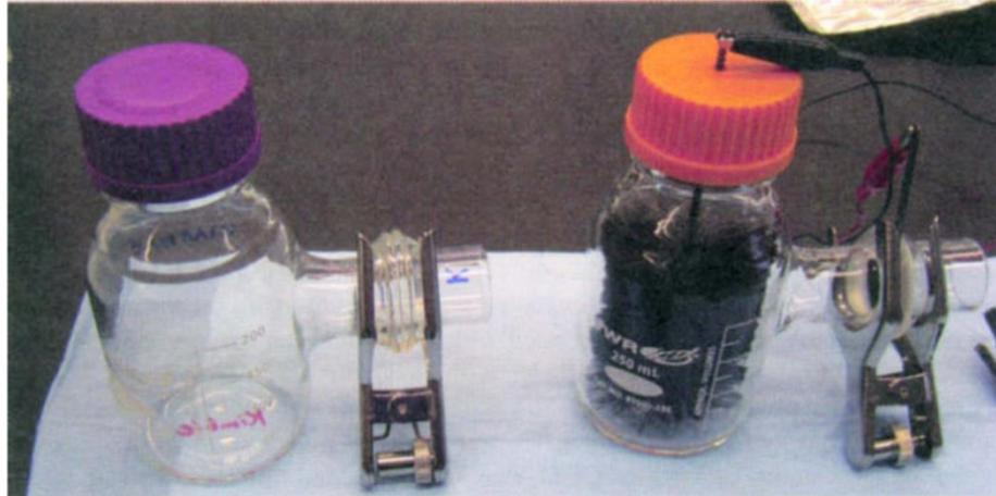
**Figure 20** Bottle shaped MFC with air-breathing cathode [100]
