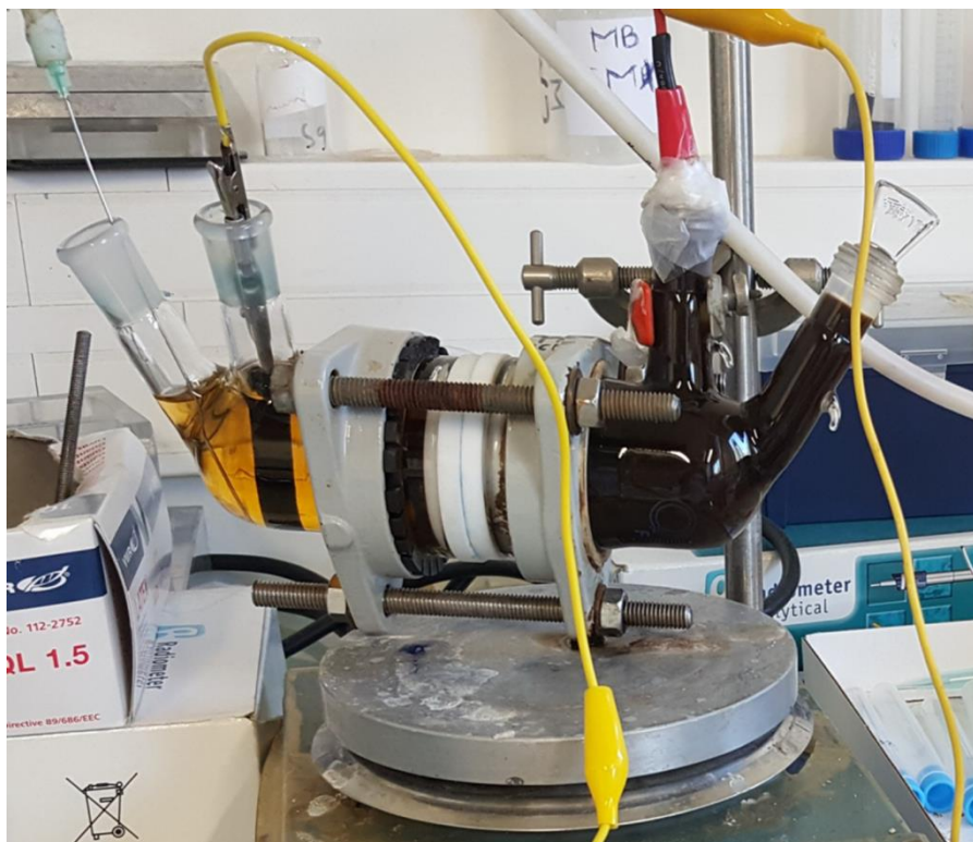
Figure-A5.1 Coupling MFC with electro-Fenton like process for degradation azo dye compound
