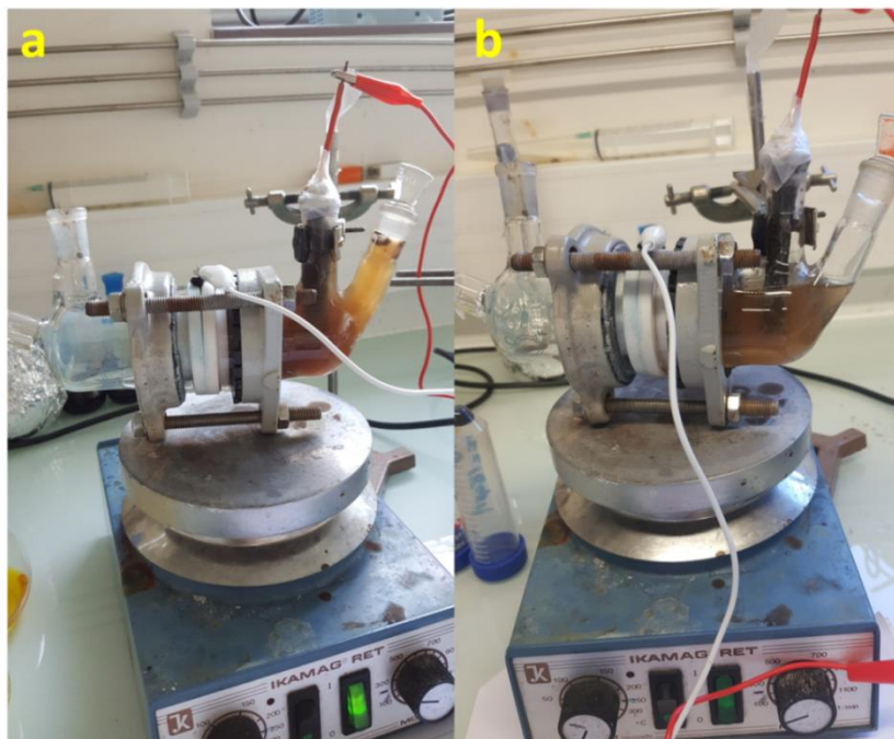
Figure 115 SCMFC operation with anodic compartment contain garden compost leachate (a) before and (b) after separation
