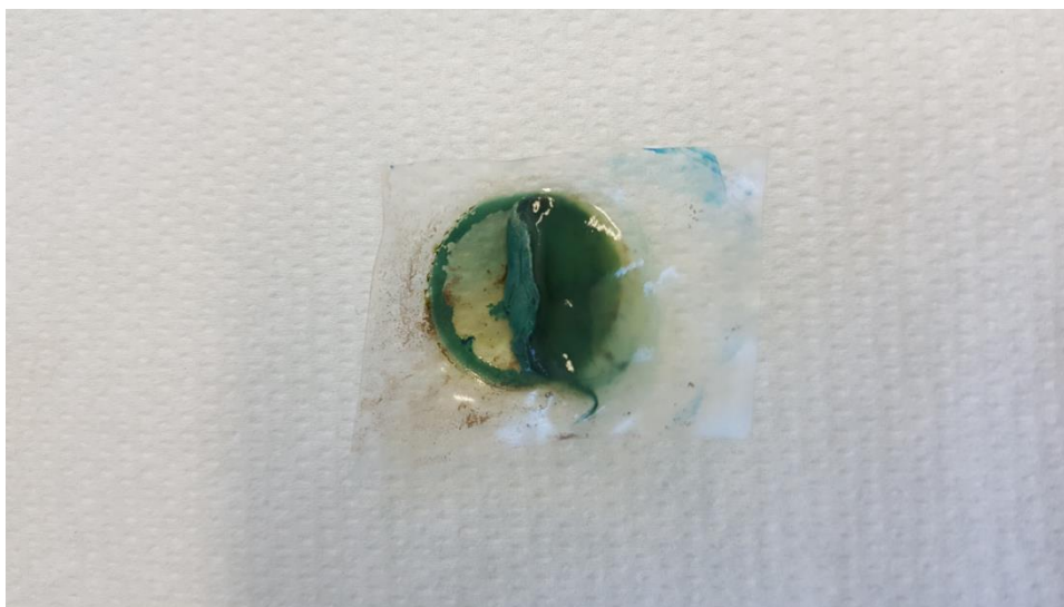
Figure-A3 Fouling found on the membrane surface which faces cathodic solution (ferricyanide) at the end of DCMFC operation
