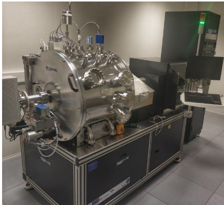
Figure 2-10 Planetary Etch System (PSIBE) from 4wave.
