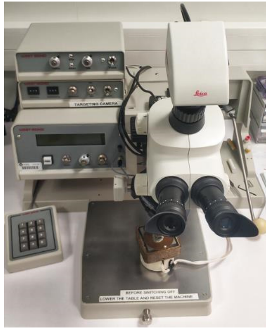
Figure 2-31 The wire bonding machine from WESTBOND.
