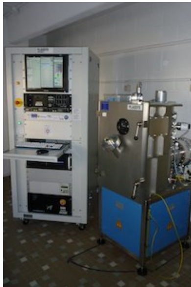
Figure 2-11 Electron beam evaporation system MEB400s from PLASSYS.
