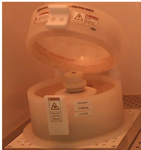
Figure 2-8 Spin coater SPIN150 from SPINCOATING.
