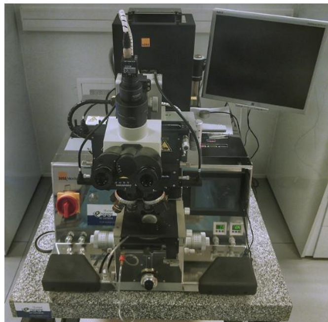
Figure 2-7 UV lithography mask aligner MJB4 from SUSS MicroTec.
