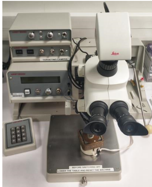
Figure 2-31 The wire bonding machine from WESTBOND.
