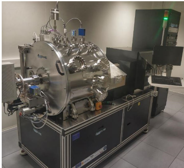
Figure 2-10 Planetary Etch System (PSIBE) from 4wave.
