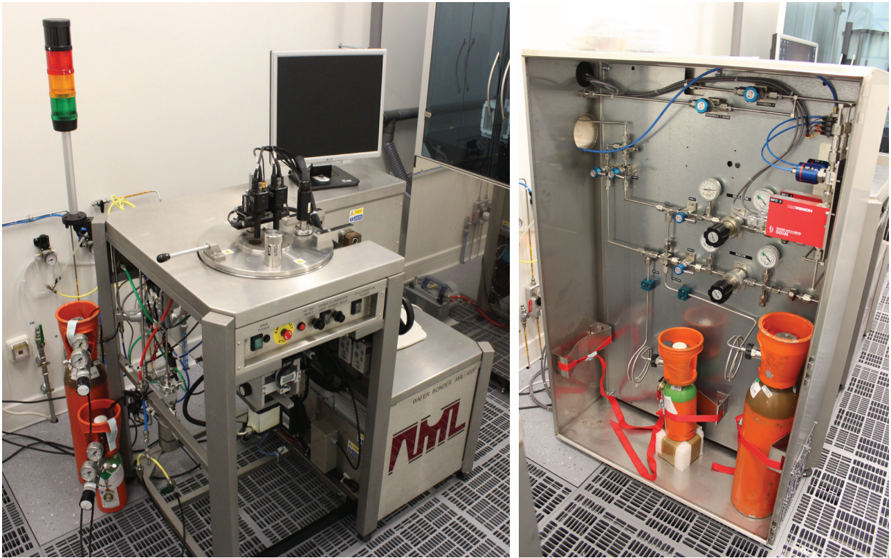
Figure 3.8: Pictures of the AML anodic bonding equipment without gas lines (left) and the dedicated gas lines added thereafter (right).
