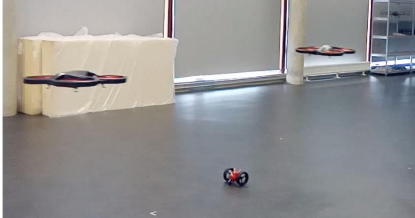
FIGURE 5.21: Experimental set for circular UAV-UGV tracking, a UGV is set as a target for two quadrotors
