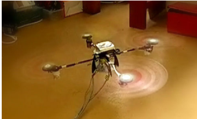
FIGURE 1.9: Quadrotor experimental setup for testing quaternion-based control algorithms proposed in [57].
