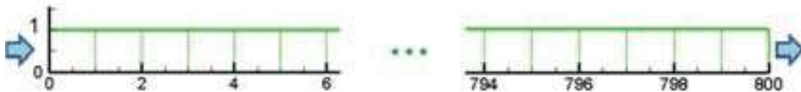
Figure 6.1 – Schematization of spatial discretization in TRACES: although the domain is 1D, solution through finite elements requires surfaces. 800 square cells of 1 \text{ m}^2 each represent the domain.
