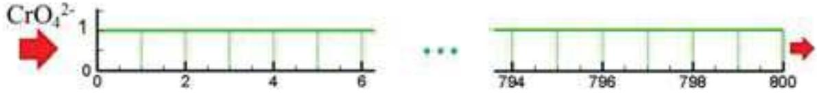
Figure 6.2 – Cr(IV) under the form of CrO4<sup>2-</sup> is absent in the domain, it is injected at the inlet and reduced to Cr(III) throughout the domain.
