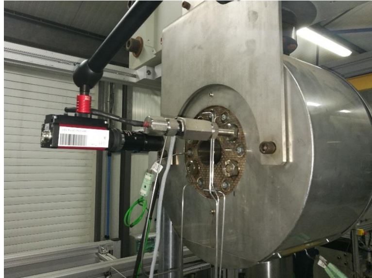
Figure 2 - 13 Camera set-up in the back side of Hycomat test bench for the marker tracking method.
