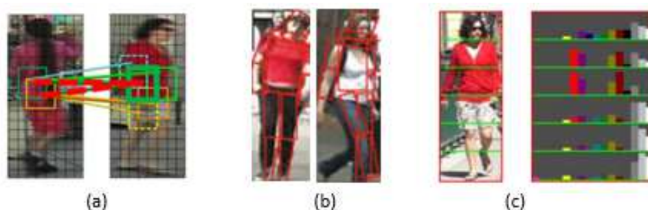
Figure 8.3: Illustrations of representative approaches of three feature extraction strategies. (a) Patch-based descriptors extracted from a dense grid [337]. (b) Descriptors extracted from segmented body parts [118]. (c) Stripe-based descriptors extracted from horizontal bands [416].
