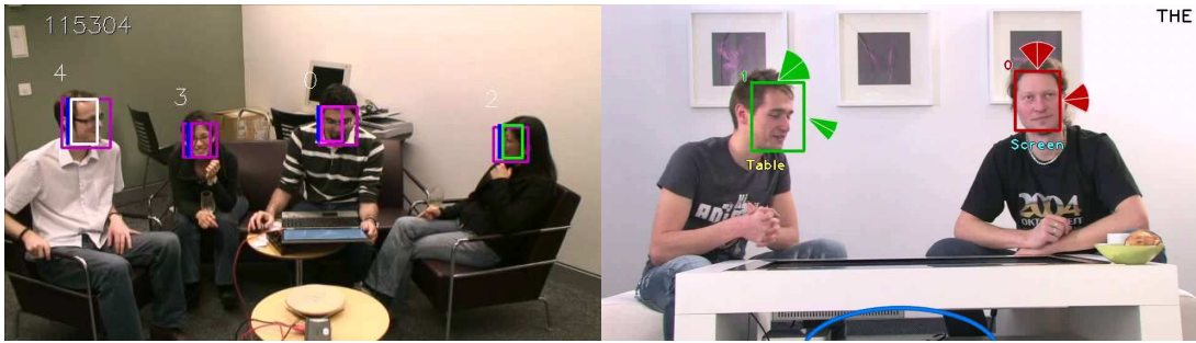
Figure 4.2: Real-time on-line multi-face tracking in dynamic environments with an RGB camera. People may move freely in the room and leave and enter the scene. Left : The proposed algorithm tracks and re-identifies a varying number of persons over long time periods despite frequent false detections and missing detections. Right : integration in a multi-modal person and speaker tracking and identification system.
