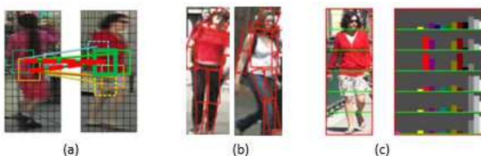
Figure 8.3: Illustrations of representative approaches of three feature extraction strategies. (a) Patch-based descriptors extracted from a dense grid [337]. (b) Descriptors extracted from segmented body parts [118]. (c) Stripe-based descriptors extracted from horizontal bands [416].
