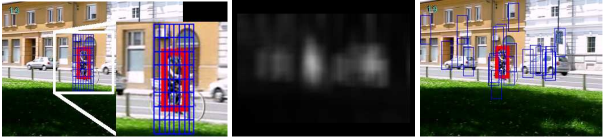
Figure 6.6: Illustration of different sampling strategies of negative examples (blue). Left : traditional sampling at fixed positions within a search window (red). Middle : the motion probability density function m (Eq. 6.11). Right : the proposed negative sampling from m .
