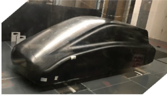
Figure 3.1: The smooth vehicle inside the working section of the wind tunnel.
