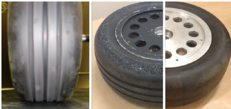
Figure 5.10: Three types of tires investigated in the study. From left to right: the reference tire having three longitudinal grooves; the reference tire with additional carborundum powder glued on the flank; the slick tire.
