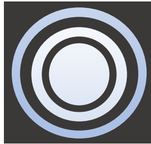
Figure 20. A circular aperture of Airy pattern in central Airy disk.
