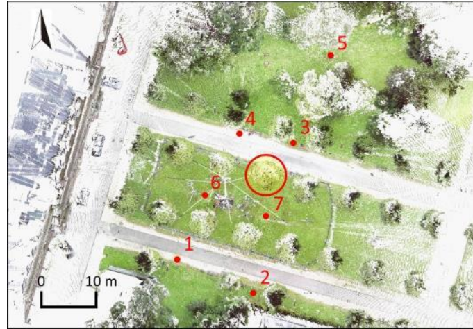
Fig. 4.3 Overview of the studied tree (red circle) and the seven TLS stations in June 27, 2016
