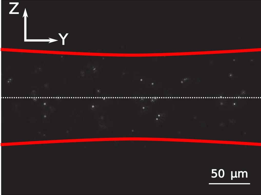
**Figure 2.4** – Example of an image recorded by our dark field microscope. The red lines highlight the contour of the laser beam and the dashed line indicate the optical axis. Each spot is a diffraction limited image of one particle. The depth of field of our imaging system is  $11.2\mu\text{m}$ . When the particle is leaving the focal volume, higher diffraction orders appear and the scattered intensity is reduced.
