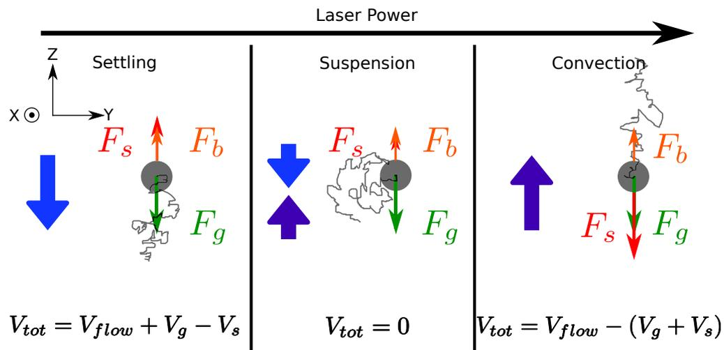
**Figure 3.2** – Applied force analysis on a single particle :  $F_b$  buoyancy force,  $F_g$  gravity force,  $F_s$  Stokes force. The blue arrow represents the settling flow direction, and the purple arrow represents the induced convective flow. From left to right :
