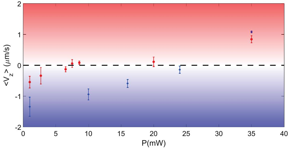
**Figure 3.14** – The suspension power for melamine beads is greater than the one needed to suspend polystyrene beads. The red dots and the blue stars are the measured velocities for polystyrene and Melamine respectively, and the error bars represents the standard error with a confidence interval of 0.95%.
