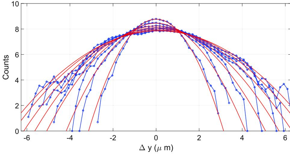
**Figure 5.6** – Displacements distributions  $\mathcal{P}(\Delta y, t)$  of the anomalous trajectories for different times  $t = \{0.5\text{s}, 1\text{s}, 1.5\text{s}, 2\text{s}, 2.5\text{s}, 3\text{s}\}$ . Remarkably the distributions remain Gaussian at all time. The counts are the number of times that the displacement of the particle lies within a given bin width of  $0.17\mu\text{m}$ .
