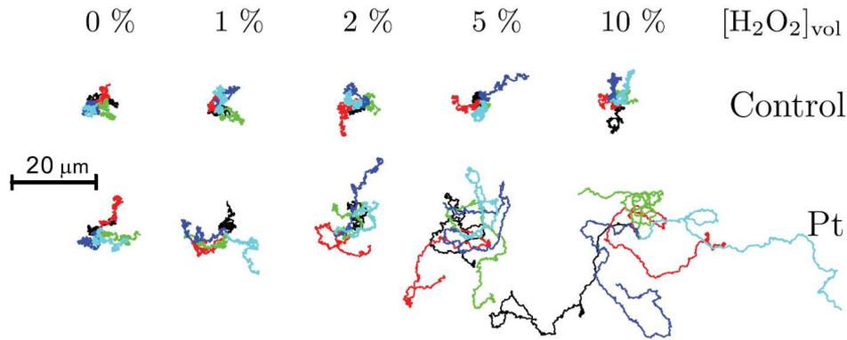
**Figure 6.2** – Example of active Janus spherical particles (Platinum-Polystyrene) trajectories. The active motion is fuelled by asymmetric catalysis of hydrogen peroxide of platinum at the surface of the half coated particles. At short time scales the motion is directed and at long time scales the motion is randomized. As shown, for non coated particles the motion is freely diffusive. However, the motion of platinum coated particles is clearly directed. This figure is directly taken from [87].
