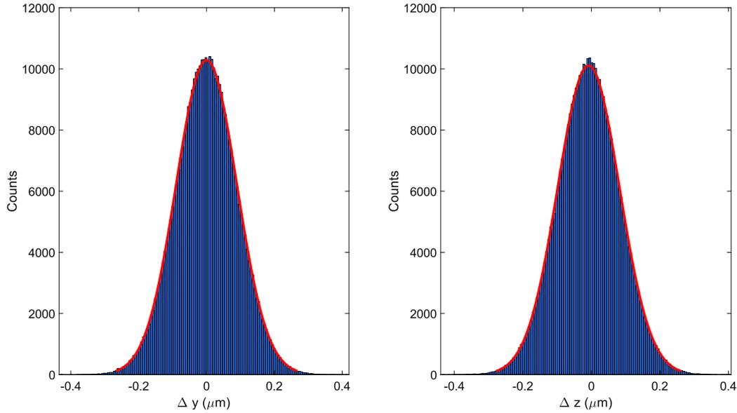
**Figure 3.10** – Distribution of all detected displacement for MI beads at  $P = 1$  mW. The total number of points used to compute the distribution is  $N_{\text{tot}} = \sum_i N_i = 4.10^5$  displacements. The histograms are constructed as presented in the methods section in chapter I. The red continuous line is a Gaussian fit of the PDF.
