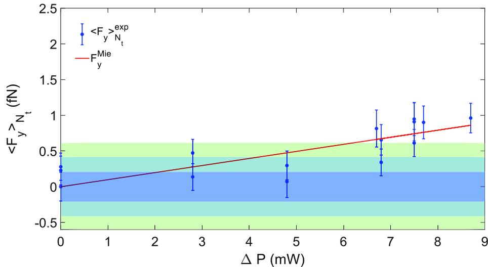
**Figure 4.21** – Mean radiation pressure force on Melamine beads along the optical axis. The errorbars represent the standard error around the mean measured force along Y. The thermal limit is calculated from equation (4.44) and displayed as  $1\sigma$ ,  $2\sigma$  and  $3\sigma$  confidence levels.
