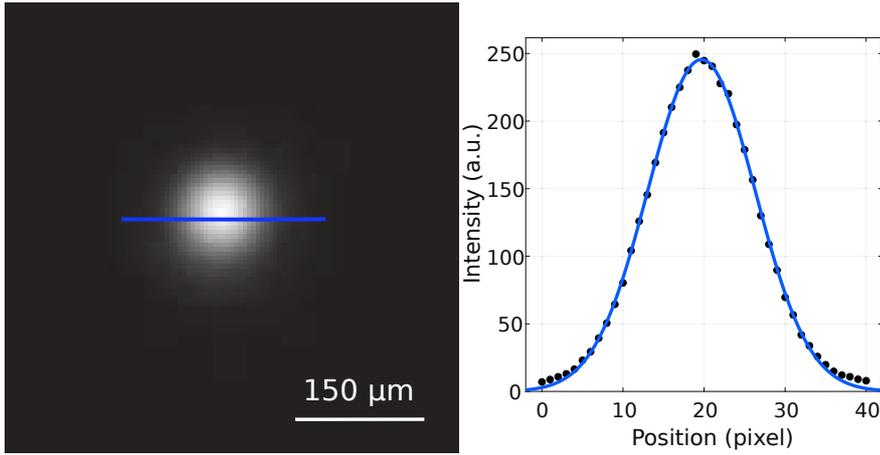
**Figure 4.22** – Direct image of the beam at the level of the sample. The pixel size of the camera we used is  $5.6 \mu\text{m}$ . We see clearly the Gaussian profile. The blue continuous line is a Gaussian fit using the Gaussian model.
