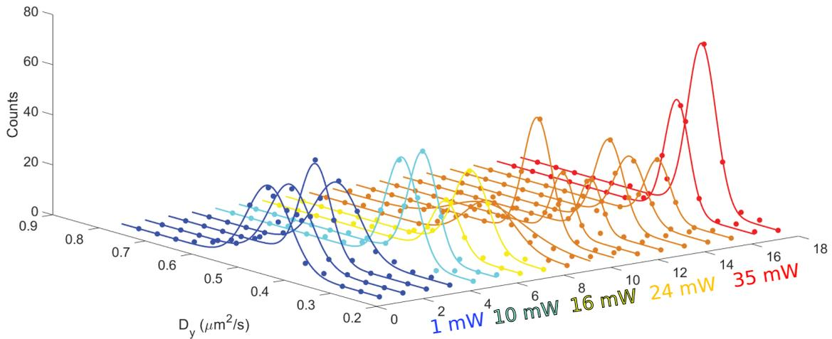
**Figure 3.12** – PDF diffusion coefficient along  $y$  for different experiments. The numbers of bins used to present the distributions is determined by the Rice rule define chapter I. The counts as presented in the methods section is the number of times we count a diffusion coefficient within the intervals defined by the bin width.
