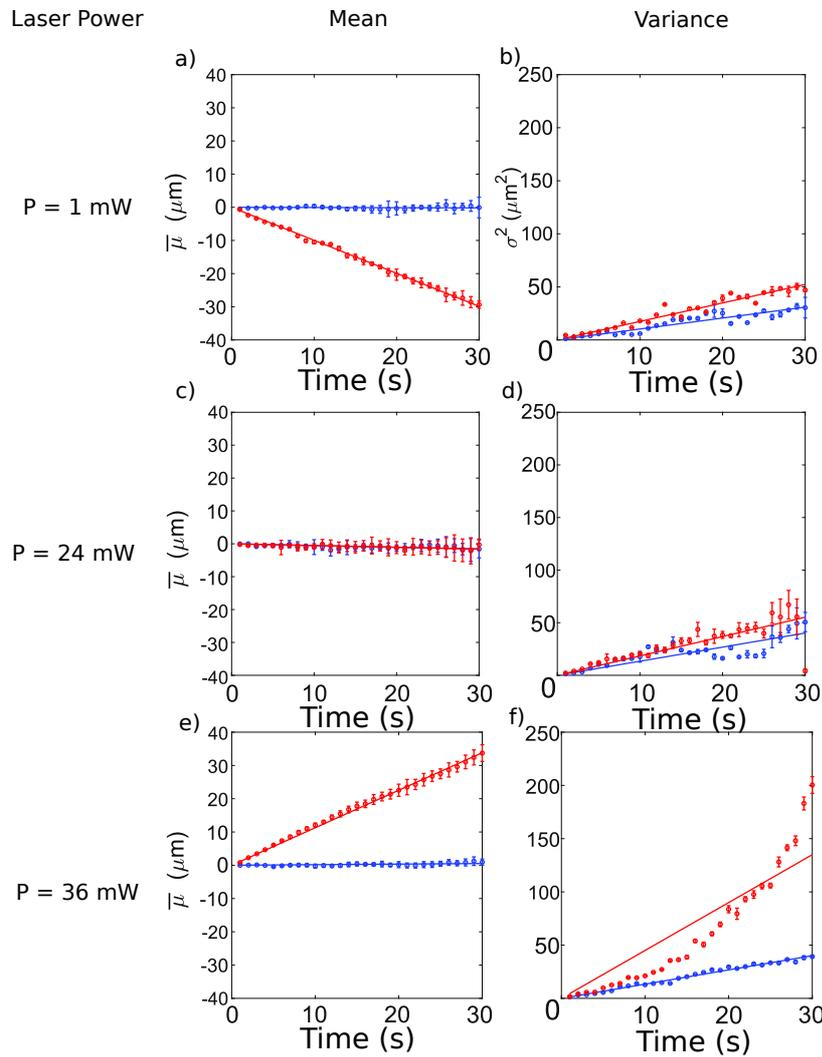
**Figure 4.7** – Evolution of the mean and the variance of the PDF of position with respect to time. The blue and red curves represents Y and Z respectively. The solid line are the fitting of the data using a linear model. The errorbars represents the confidence intervals at 95% computed from fitting the PDFs
