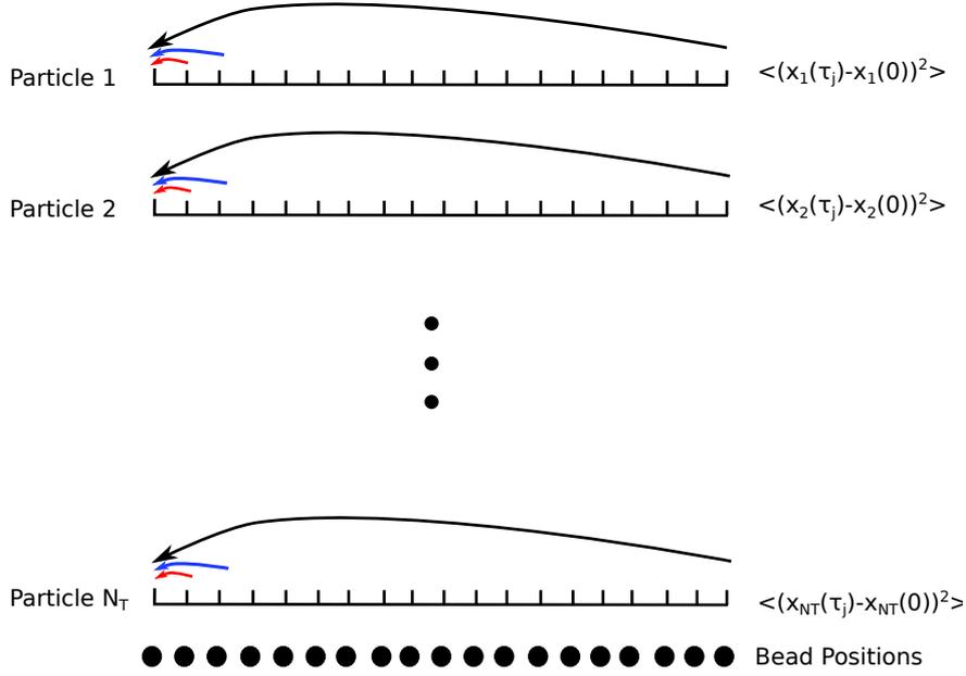
Figure 4.13 – Procedure to calculate the EAMSD.
