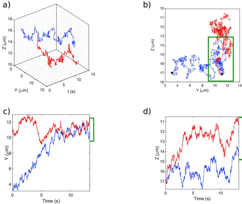
**Figure 5.4** – Example of recorded trajectories of two interacting Melamine particles. Panel (a) displays the evolution of the 2D trajectories with respect to time. In panel (b) the 2D trajectories are presented. The panel (c) and (d) are the 1D projections of the interacting particles. The confinement is highlighted by the green rectangle and the corresponding regions are showed in panel c) and d).
