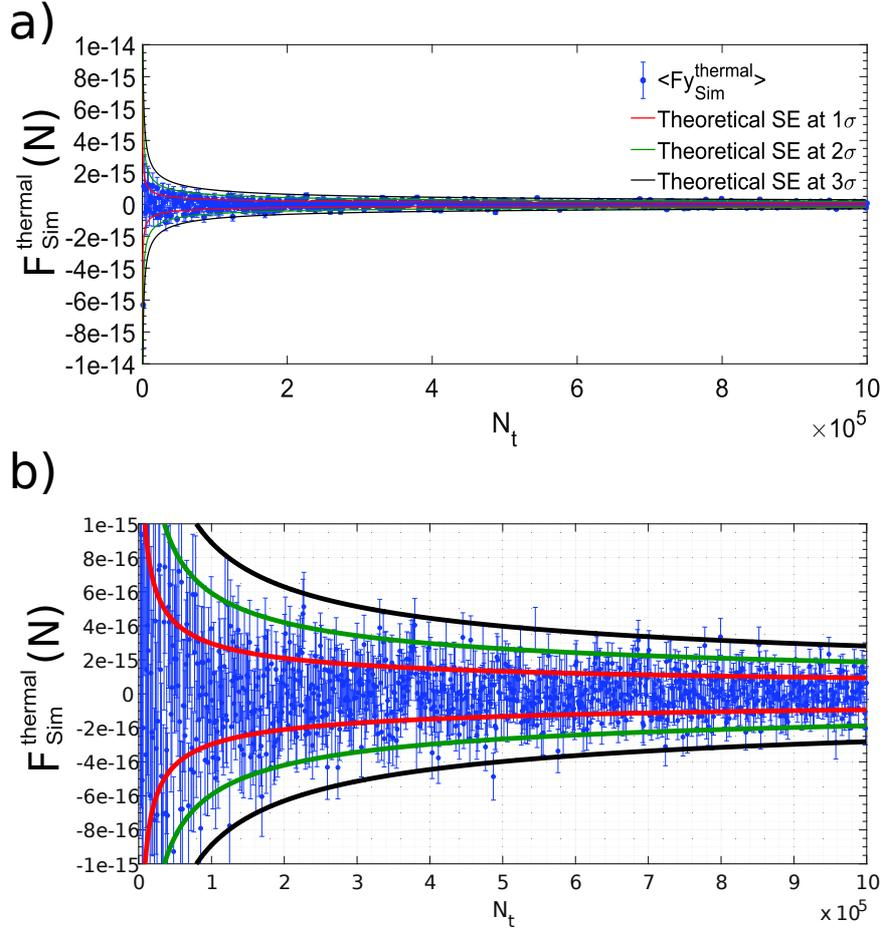
**Figure 4.17** – Mean thermal force  $F_{Sim}^{thermal}$  extracted from simulated trajectories as the sample size  $N_t$  (total number of simulated displacements) increases. The errorbars are the standard errors defined (4.42). Panel (b) is a zoom of panel (a) in the small sample limit.
