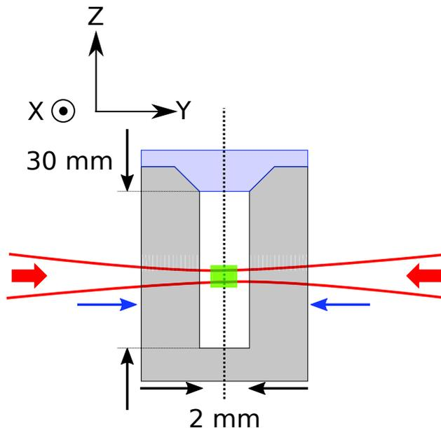
**Figure 3.1** – Experimental SetUp in the contra propagating scheme. The red arrows represents the direction of propagation of each beam, the blue arrows is the confocal parameter which is in the experiment  $2Y_R = 12\text{mm}$ . The green area is the field of view of our microscope  $350\mu\text{m} \times 250\mu\text{m}$ . For our measurements we use Melamine bead with a diameter  $d = 940\text{ nm}$ .
