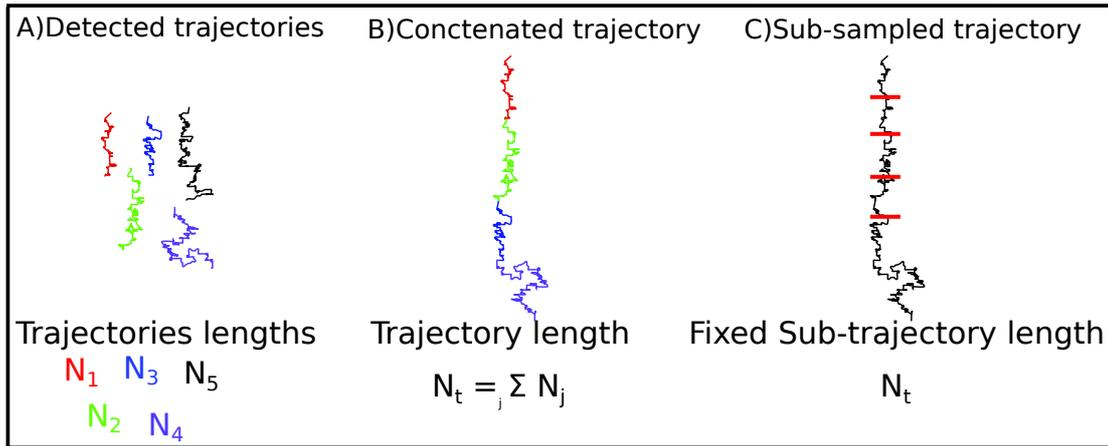
**Figure 4.4** – Sketch of the concatenation strategy starting from individual trajectories first, we link the tracked trajectories as shown in panel b). Then, for a chosen time delay  $T_{\text{sub}}$  we divide the concatenated trajectory into equal trajectories. The number of sub trajectories is by construction defined from the ratio between the total duration of the concatenated trajectory and  $T_{\text{sub}}$ .
