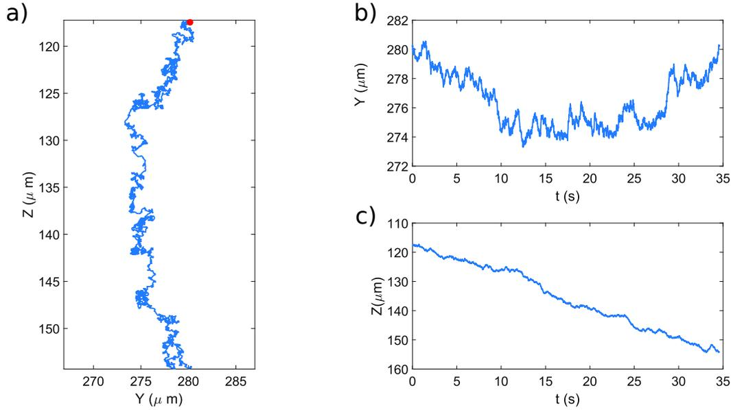
**Figure 2.10** – Recorded trajectory of a Melamine bead sedimenting in water. Panel a) shows the 2 D trajectory where the red dot representing the initial positions recorded at  $t=0$ . Panels b) and c) are the projection along  $Y$  and  $Z$  axis.
