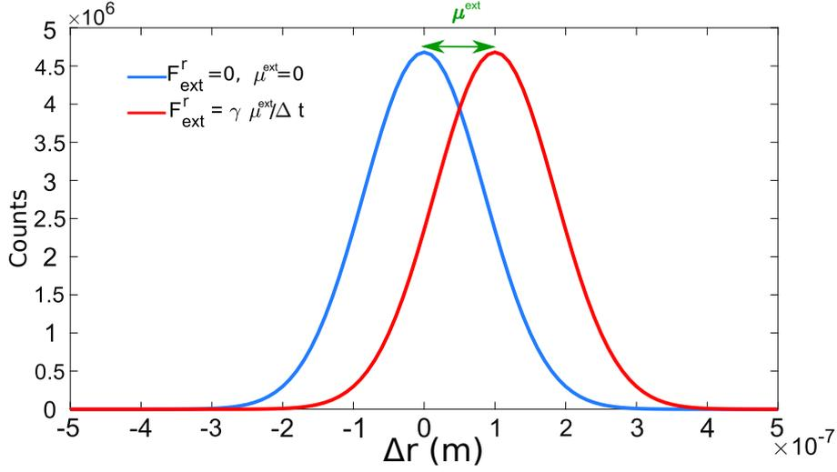
**Figure 4.2** – Simulated Displacement distribution  $P(\Delta r, \Delta t)$  for a Brownian particle. Blue line : free Brownian motion without external force, red line : Brownian motion under an external force  $F_{\text{ext}}$  directed along  $r$ , with the corresponding  $\mu^{\text{ext}}$  ballistic shift.
