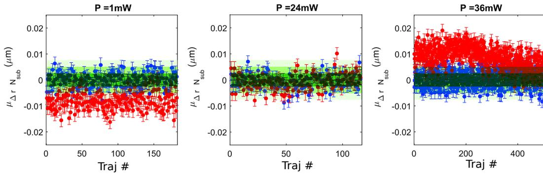
**Figure 4.8** – Estimators of the mean displacement of the sampled trajectories. The blue and red bullets represents respectively the Y and Z directions. The green shaded region represents standard error from mean theoretical displacement due to thermal fluctuations : from the darker to the lighter green  $1\sigma$ ,  $2\sigma$ , and  $3\sigma$  confidence levels.
