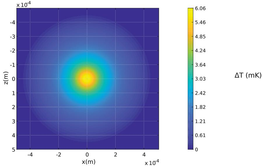
**Figure 3.18** – Temperature change profile map in the  $(\vec{e}_x, \vec{e}_z)$  plane for a laser power  $P_0= 35 \text{ mW}$ , taking the absorption of water at  $\lambda_L = 637 \text{ nm}$ .
