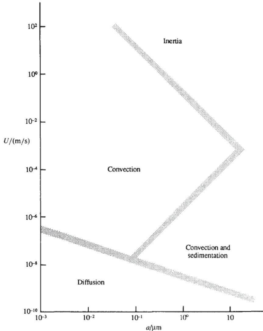
**Figure 1.4** – Dominant mechanism in colloidal suspensions depending on the size  $a$  and the velocity  $U$  of the colloidal particle. In our experiments the typical velocities are in the order of  $U \sim 1 \mu m s^{-1}$  and the particle size is  $a \sim 0.5 \mu m$ . This figure is taken from [33].
