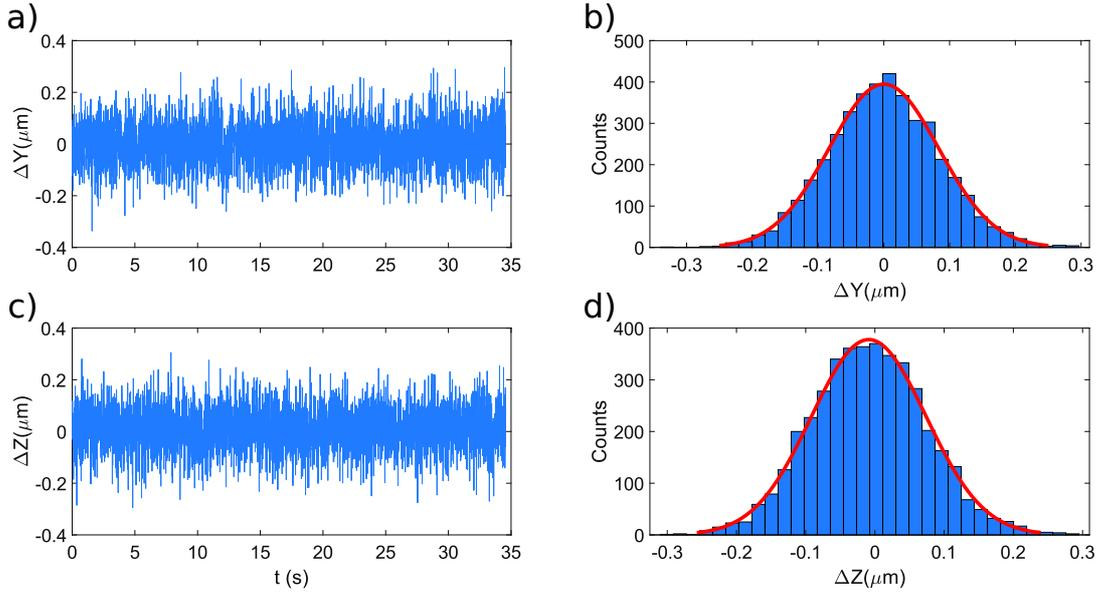
**Figure 2.11** – Constructed PDF of displacements of the trajectory presented in (2.10). Panels a) and c) shows respectively the temporal displacements along the Y and Z axis. The panels b) and d) represents the PDFs of displacements constructed using the method described in the main text.
