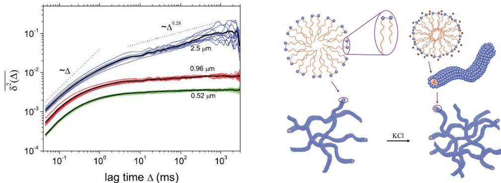
**Figure 5.2** – Time Averaged MSDs for a mixture of micelles and polystyrene beads of different diameters  $\{0.52\mu\text{m}, 0.96\mu\text{m}, 2.5\mu\text{m}\}$ , where  $\Delta$  is the time lag over which the squared displacements are averaged. The black line represent the ETA-MSD defined by equation (3.10). The data are taken from [73]. The right hand side displays the micellar solution used in the experiment of [79] with added polystyrene beads.
