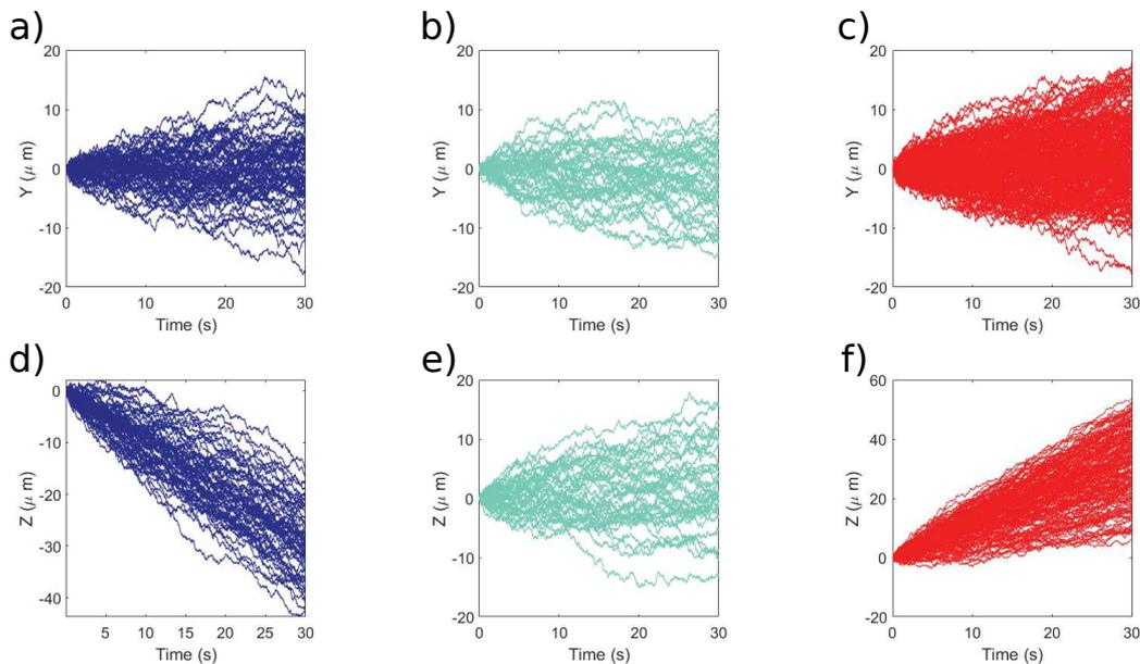
**Figure 4.5** – 1D sub-trajectories along Y and Z axes, corresponding to the trajectories displayed in figure (4.3). The drift seen in panels d) and f) is induced by sedimentation and convective flow respectively. The free Brownian character of the suspended regime is clearly seen in panels b) and e). The number of sub-sampled trajectories for the sedimentation, suspension and convective regimes are respectively 61, 39 and 169.
