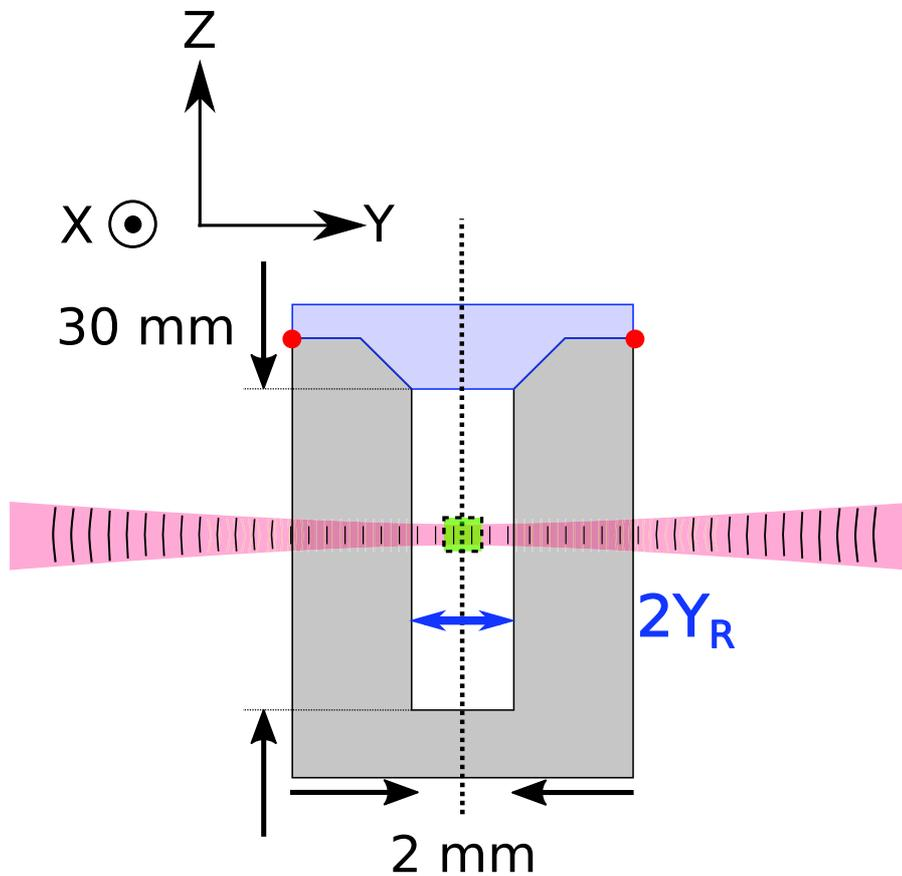
**Figure 2.3** – Sketch of the sample cell. The cell is a "spectroscopic cell" (purchased at Hellma Analytics) made of optical glass with four windows. The dimensions are : height 45 mm, width 12.5 mm and depth 12.5 mm. The dimensions inside of the cuvette are 30 mm height, 2 mm width and 10 mm depth. The red dots represent the vacuum grease sealing. The blue segment shows the confocal parameter. F.O.V is the field of view of the dark field microscope.
