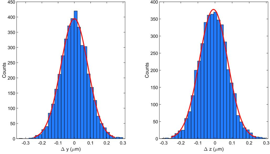
**Figure 3.11** – Distribution of displacements for one M1 bead at  $P = 1$  mW. The red continuous line is a Gaussian fit of the PDF. The total number of points used to compute the distribution is  $N_i = 4150$ .
