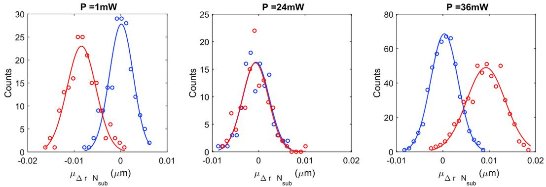
**Figure 4.9** – PDF of the mean displacement of the sub sampled trajectories. The continuous lines represents a normal fit to the distribution of the mean of the estimator of the mean displacement for each sub-trajectory. The distributions are clearly sharp around the mean displacement. The counts are the number of estimated means that falls within the bin width defined in chapter I.
