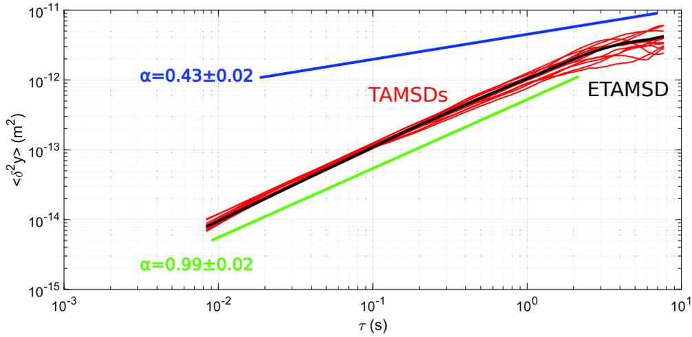
**Figure 5.5** – The red curves are the TAMSDs  $\delta_r^2(\tau)$  of 12 anomalous trajectories detected for an experiment recorded over 90 min. The black line is the ETAMSD  $\langle \delta_r^2(\tau) \rangle$  of the ensemble of anomalous trajectories. The blue line represents the exponent of the fitted ETAMSD which is  $\alpha = 0.43 \pm 0.02$  for long time. The green line represents the fitted ETAMSD for short time :  $\alpha = 0.99 \pm 0.02$ .
