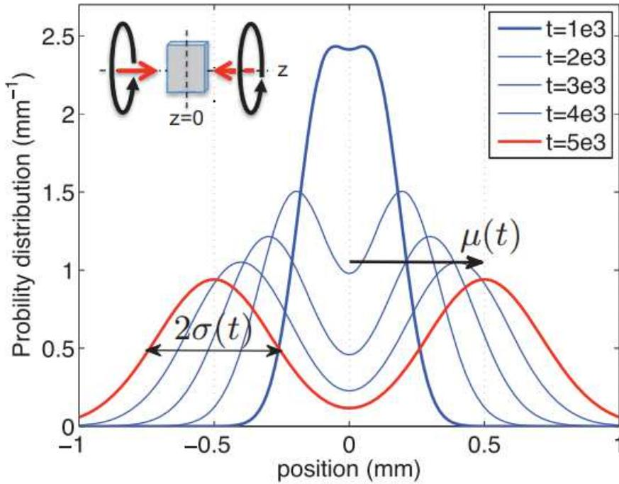
**Figure 6.1** – Demonstration of chiral particles separation induced by dissipative chiral forces. A racemic mixture illuminated by counter-propagating circularly polarized two-beam configuration, can be sorted. A separation of 1 mm is predicted for an experiment lasting one hour. This figure is from [16].
