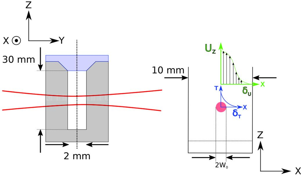
**Figure 3.16** – Left hand side : front view of the sample, with the dimensions :  $L_x = 10\text{mm}$ ,  $L_y = 2\text{mm}$ ,  $L_z = 30\text{mm}$ . Right hand side : Cross cut in the  $(XZ)$  plan,  $W_0 = 50\mu\text{m}$  is the beam waist with a Rayleigh length  $Y_R = 12\text{mm}$ , and  $\delta_T$  and  $\delta_u$  are the thermal and velocity boundary layers respectively.
