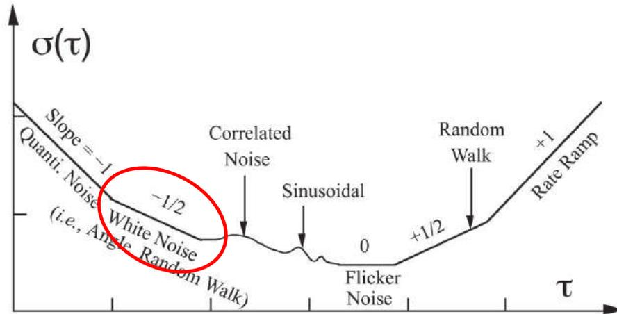
**Figure 4.18** – Sample plot of AV analysis [68] for different sources of noise. The slope of AV gives what type of noise and over which time window this noise determines the studied process.
