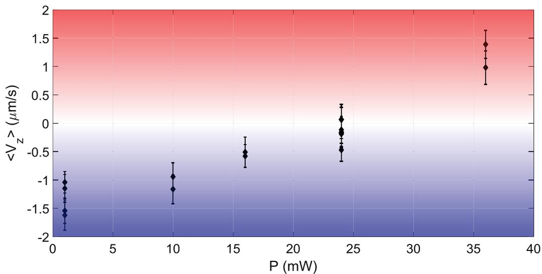
**Figure 3.5** – Mean velocity along the  $z$ -axis for different laser power  $P_0$  for 1  $\mu\text{m}$  melamine beads. The blue region is the sedimentation regime, the green region is the convective regime, and the white region is the suspension regime. The errorbars are the standard deviation around the estimator of the mean velocity.
