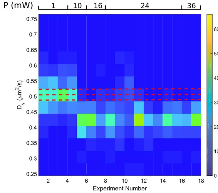
**Figure 3.13** – Color map of PDF diffusion coefficient along  $y$  for different experiments. The red dashed line are the theoretical diffusion coefficient calculated from Stokes Einstein relation taking into account the size dispersion.
