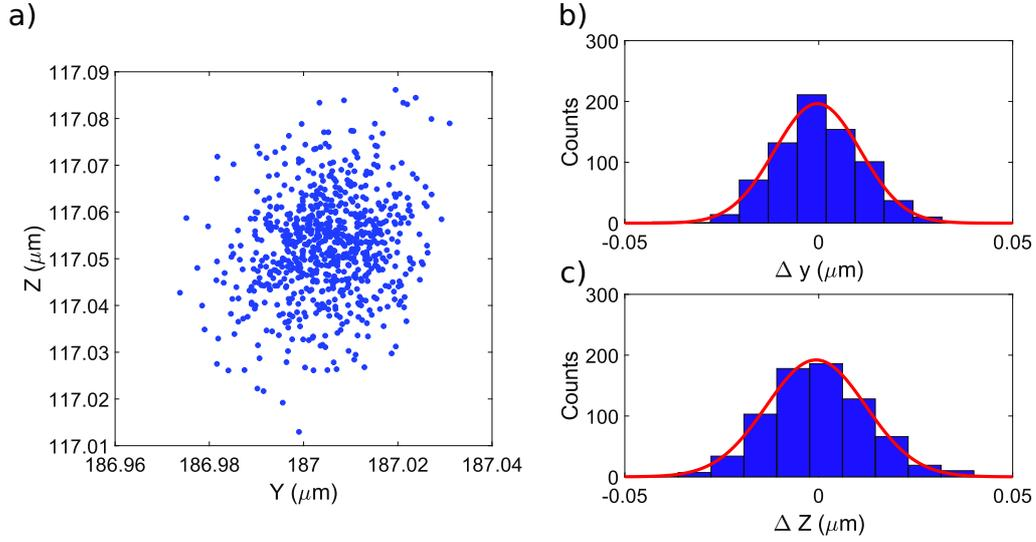
**Figure 2.7** – (a) Tracked positions of a fixed bead. Panels (b) and (c) shows respectively the displacement histogram along Y and Z directions. The counts are the number of times that the displacement lies within the bin width which is in this case 7 nm. The localisation uncertainties are given by the width of the distribution :  $\sigma_0^y = 8 \pm 1 \text{ nm}$  and  $\sigma_0^z = 9 \pm 0.5 \text{ nm}$ .
