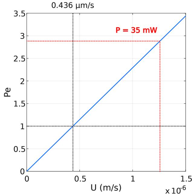
**Figure 3.21** – Dependence of Peclet number on the flow velocity. When the flow velocity exceeds  $0.436 \mu\text{m/s}$ , the advective motion starts dominating over the the diffusive motion. The red dotted line correspond to our experimental regime of induced convection with  $P_{High} = 35 \text{ mW}$
