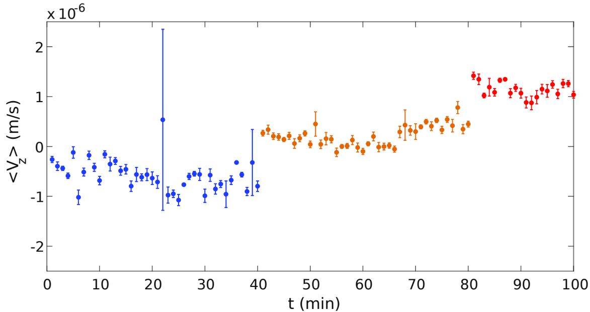
**Figure 3.15** – Evolution of the estimator of the mean vertical velocity of polystyrene beads of radius  $R = 0.5\mu\text{m}$ . Each data point represents the mean velocity averaged over the mean displacements detected during one minute. The error bars are the standard deviation around the mean velocity. The blue, orange and red colors represents laser powers at 1 mW, 8 mW and 35 mW respectively.
