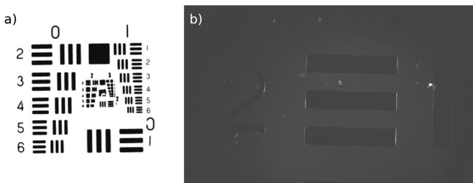
**Figure 2.6** – Calibration target used for the determination of the pixel size of our imaging system. Panel (a) shows the calibration target and in panel (b) an image recorded by the microscope is displayed.
