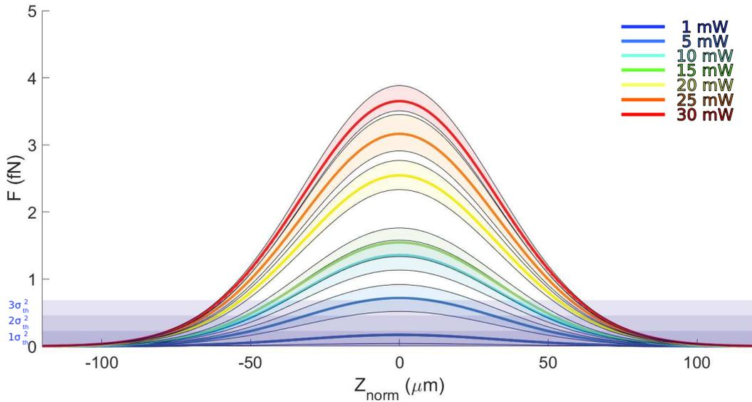
**Figure 4.23** – Reconstructed force profiles for different laser power. The shaded regions represents the confidence intervals at 95%. The uncertainties displayed around the reconstructed profile are the SE defined in equation (2.41).
