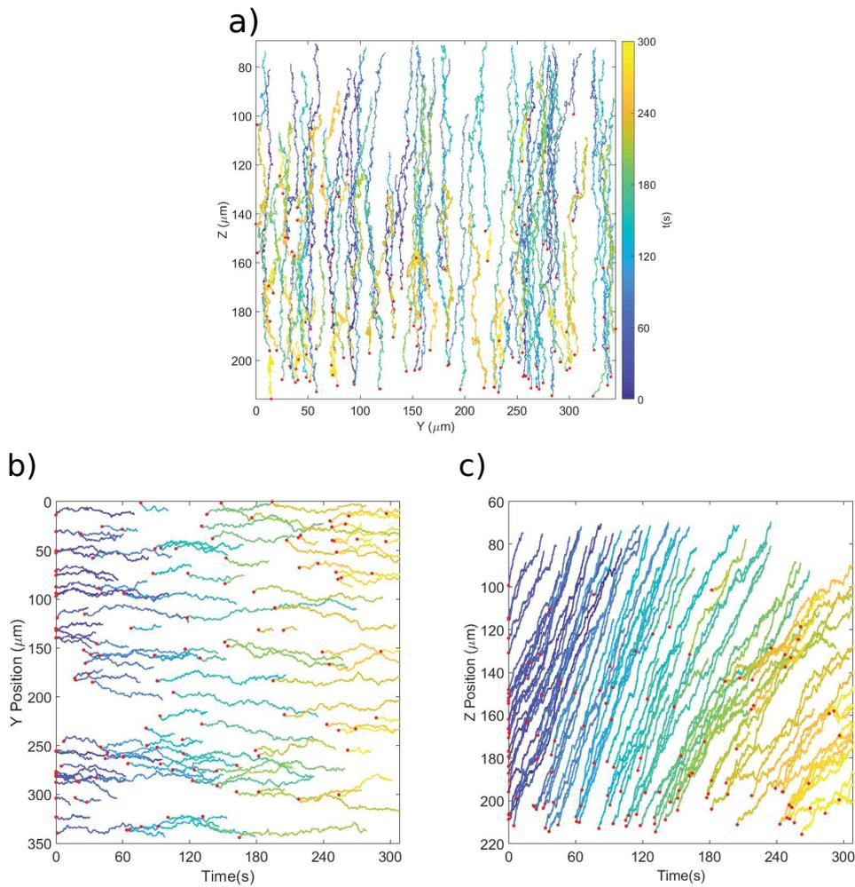
**Figure 3.4** – Tracked trajectories of Melamine particles with radius  $R = 0.47\mu\text{m}$  at high laser power : panel a) trajectories in the Y-Z plan, panels b) projection along Y axis where the motion is still diffusive and panel c) projection along the Z axis where the motion is ballistic and directed upward. The color bar represents the time when we start tracking the particle.
