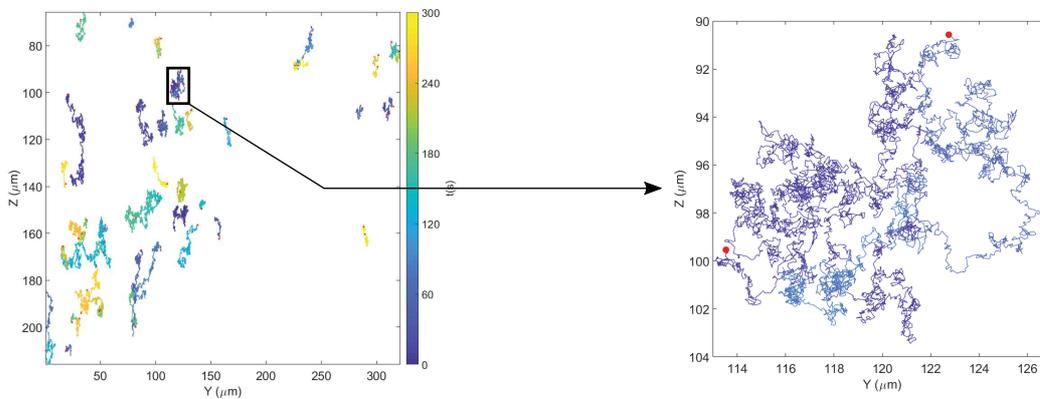
**Figure 3.6** – Tracked trajectories of Melamine particles with radius  $R = 0.47\mu\text{m}$  at a laser power  $P = 24$  mW. In the right hand side a zoom is presented to displays the "Free Brownian motion" character of the suspended regimes.
