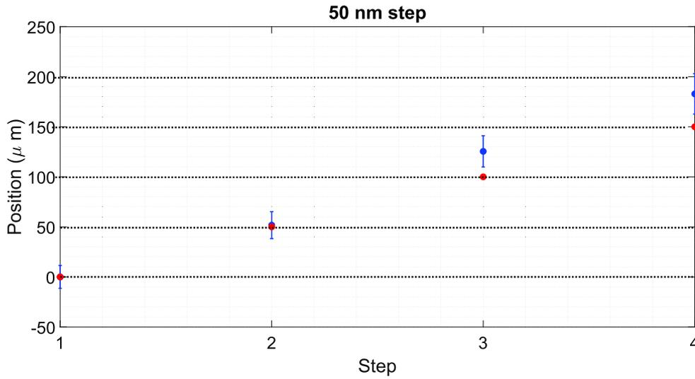
**Figure 2.8** – Displacement resolution for 50 nm step. The error bars are the standard deviations around the mean position calculated from the ensemble of displacements. There is a good agreement between the real position and the detected one for the two first points. There is an issue for the two other measurements but the difference between the two detected positions and the two real position is the same, confirming that a displacement of 50 nm is well resolved by our microscope.
