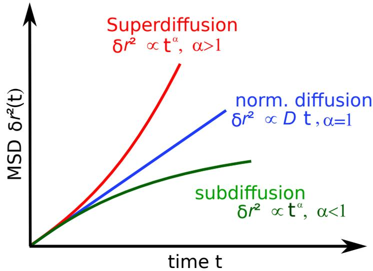
**Figure 5.1** – Time Averaged MSD for different type of dynamics. For free diffusion the TA-MSD grows linearly with respect to the time lag  $\tau$ . Sub-diffusive motion is characterized by a slower evolution of the TA-MSD. The super diffusive TA-MSD is representative of a ballistic motion due to an external flow transporting the particle, as discussed in chapters 3 and 4.
