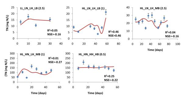
**Figure 10-2** Experimental TN data at the effluent (diamond with error bars indicating measurement uncertainty) of different modalities (graph title with best fit order in brackets) fitted to the coupled RTD and mixed-order model (line).
