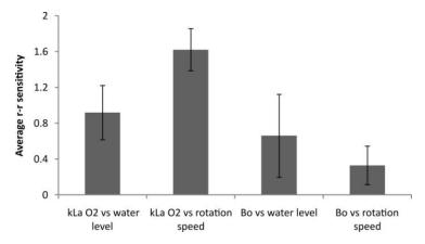
**Figure 8-5** Average Relative-Relative sensitivities (dimensionless) of oxygen transfer coefficient and Bodenstein number versus water level and paddle rotational speed. Data was converted to absolute value for comparison.
