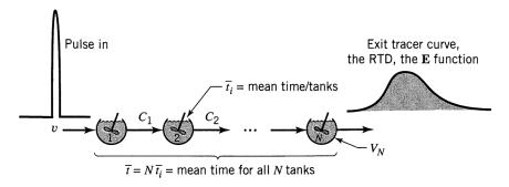
**Figure 2-4** Illustration of the Tanks-in-Series model (Levenspiel, 1999).
