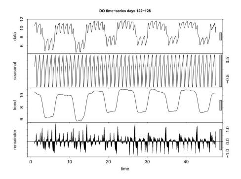
**Figure 9-4** Example of decomposition of time series D0 data (time scale in 0.125 days time-steps and D0 data in mg/L).
