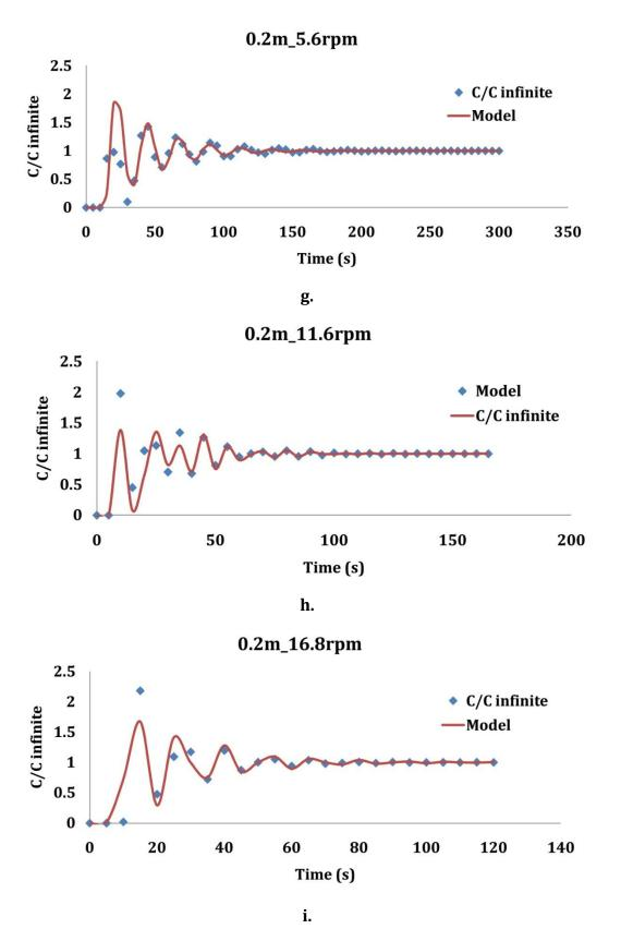
Figure A 12 Fitting curves (model vs. real data) for each mixing characteristics test.
