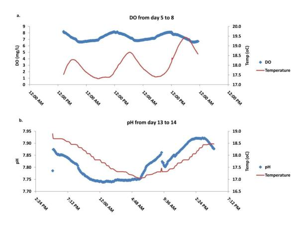
**Figure A 8** Examples of DO and pH profiles in 24h of the pilot HRAP under low light condition.
