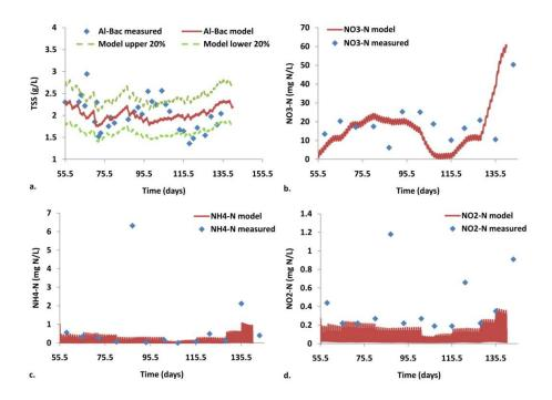
**Figure 11-2** Experimental (dots) and simulated (lines) TSS (a.), nitrate (b.), ammonium (c.), and nitrite (d.) nitrogen values in the HRAP for 85 days since the day 55. Measured TSS data was used for model calibration, 20% variation was calculated from the simulated result (a.).
