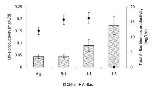
**Figure 7-1** Global Al-Bac biomass and Chl-a productivities of biomass with different initial algae/activated sludge ratios (error bars indicate standard error between fitted values and observed values).
