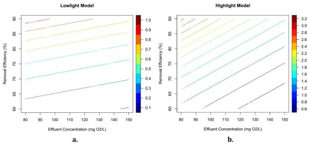
**Figure 10-5** HRAP sizing following low light (a.) and high light models (b.) with the color bar indicates mean residence required.
