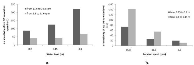
**Figure 8-4** Absolute-Relative sensitivity (d<sup>-1</sup>) of oxygen transfer coefficient (k<sub>L</sub>a<sub>02</sub>) versus paddle rotational speed (a.) and water level (b.). The sign represents positive (no sign) or negative (- sign) correlation.
