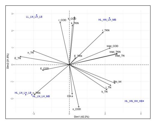
**Figure 10-4** PCA biplot showing relationships between various experimental and model parameters for different modalities. In the figure, Chl\_a and Bio\_tot refer to concentrations of Chlorophyll a and total biomass in HRAP. Inlet\_i and E\_i are the inlet concentration and average removal efficiency of substance i, respectively. While n\_i, k\_i and r\_i are optimal reaction order, reaction rate constant and reaction rate of related to removal process of substance i, respectively.
