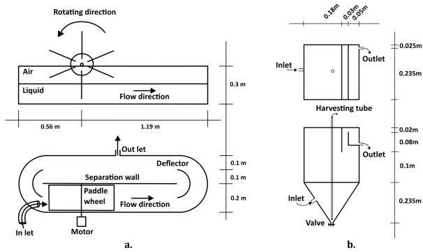
**Figure 4-4** Side view and top view of a. the pilot HRAP and b. the settler.
