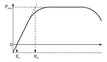
**Figure 1-5** Typical photosynthesis–irradiance response curve with  $P_{max}$  is maximum photosynthetic rate reached at saturating irradiance ( $E_k$ ) while  $E_c$  is irradiance compensation point (Barsanti and Gualtieri, 2006).
