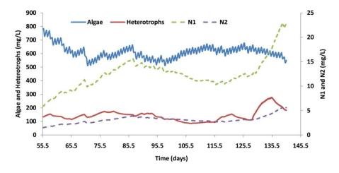
**Figure 11-6** Simulated concentrations of algae, heterotrophic, ammonium oxidizing and nitrite oxidizing bacteria in the HRAP for 85 days since the day 55.
