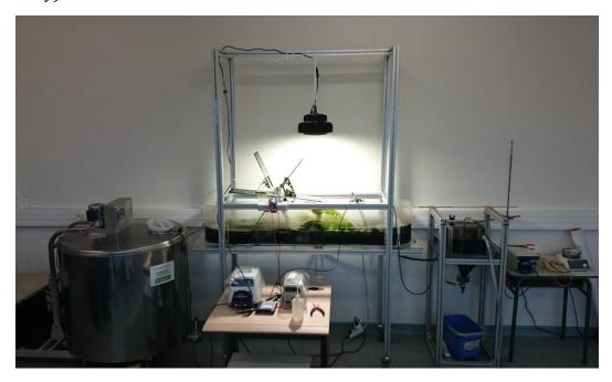
Figure A 9 HRAP system operation (high light condition).
