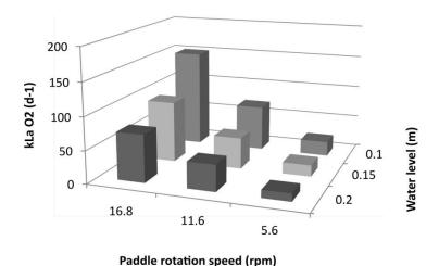
**Figure 8-3** Influence of paddle wheel rotation, water level to oxygen transfer coefficient in pilot HRAP.
