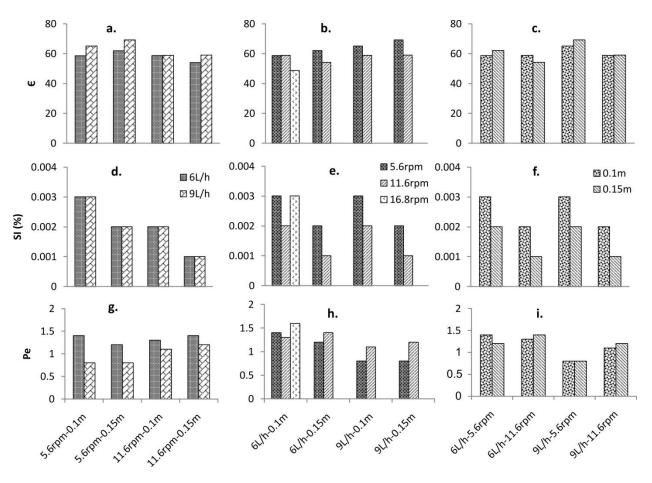
**Figure 8-6** Influence of inlet flow rate (a, d, f), paddle wheel rotation (b, e, g) and water level (c, f, h) to effective volume fraction ( $\epsilon$ : a, b, c), Short-circuiting Index (SI (%): d, e, f) and Peclet number (Pe: g, h, i) in pilot HRAP.
