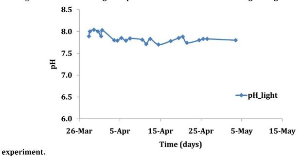
**Figure A 7** pH measured in the pilot at day time during the low light experiment.
