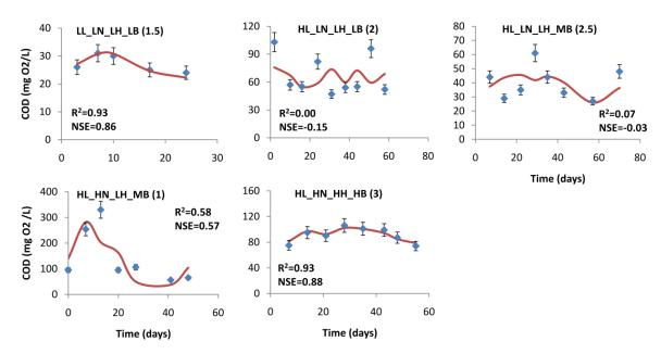
**Figure 10-1** Experimental COD data at the effluent (diamond with error bars indicating measurement uncertainty) of different modalities (graph title with best fit order in brackets) fitted to the coupled RTD and mixed-order kinetic model (line).
