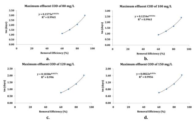
**Figure A 17** Exponential relationship between required tm and expected removal efficiency for different expected maximum effluent COD concentrations according to high light model.
