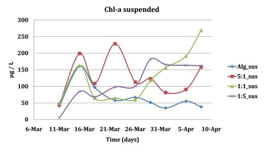
**Figure A 4** Chl-a level of aqueous phase after settling for 1h in each reactor.
