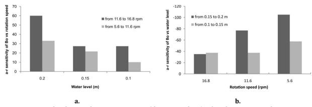
**Figure 8-2** Absolute-Relative sensitivity (dimensionless) of Bodenstein number versus paddle rotational speed (a.) and water level (b.). The sign represents positive (no sign) or negative (- sign) correlation.
