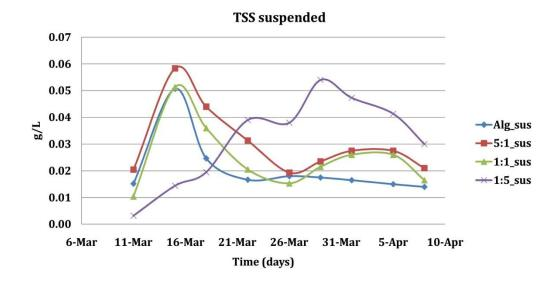
Figure A 2 TSS level of aqueous phase after settling for 1h in each reactor.
