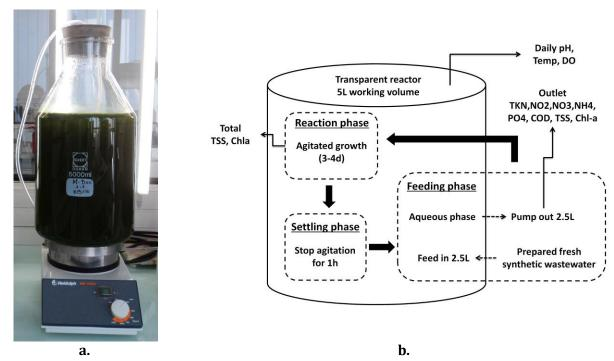
**Figure 4-3 a.** Real picture of a working reactor and **b.** Experimental protocol illustration: highlighted arrows - shifting between phases, normal arrows - biomass, physiochemical and biochemical measurements, dashed arrows – exchange aqueous phase with fresh synthetic wastewater.
