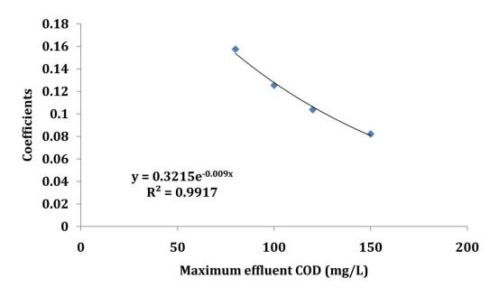
**Figure A 18** Exponential relationship of coefficients obtained above to derive the empirical law for HRAP sizing according to high light model.
