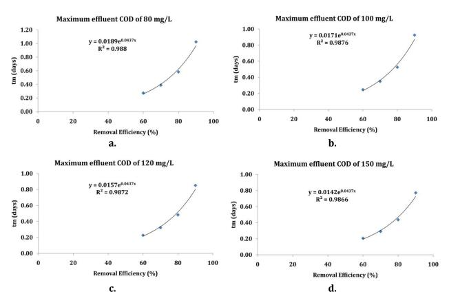
**Figure A 15** Exponential relationship between required tm and expected removal efficiency for different expected maximum effluent COD concentrations according to low light model.
