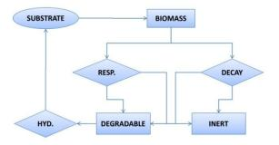
**Figure 3-3** Illustration of death-regeneration with hydrolysis.
