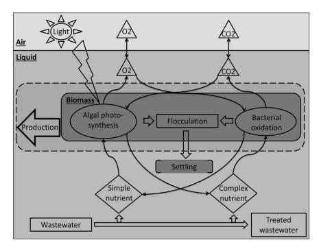
**Figure 1-1** General illustration of algal-bacterial processes in wastewater (big arrows indicate main processes, normal arrows indicate mass transferring between phases including Air, Liquid and Biomass).
