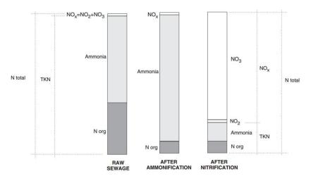
**Figure 1-3** Distribution of nitrogen in a treatment system with nitrification (Sperling, 2007).
