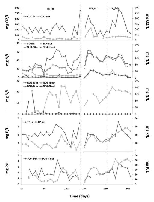
**Figure 9-1** COD, N and P concentrations at the influent and effluent of the HRAP (data of LN\_4d modality fit with left scale, data of HN\_4d and HN\_8d modalities fit with right scale).
