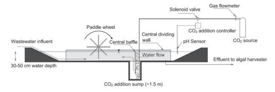
**Figure 1-2** Cross-sectional side view of a HRAP with CO<sub>2</sub> aeration (Park et al., 2010).
