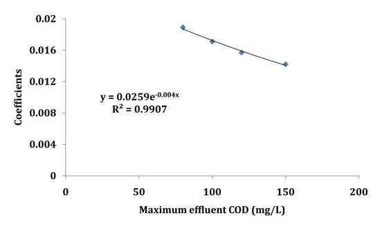
**Figure A 16** Exponential relationship of coefficients obtained above to derive the empirical law for HRAP sizing according to low light model.
