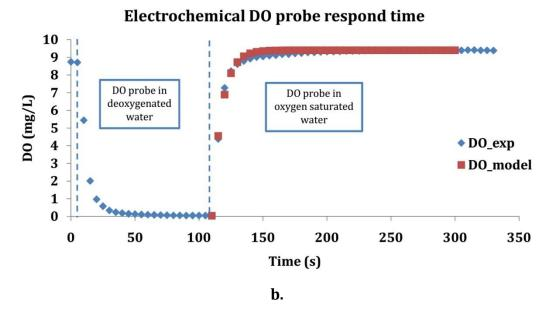
**Figure A 13** Fitting curves for **a.** optical DO probe (DO probe 1) and **b.** electrochemical DO probe (DO probe 2).
