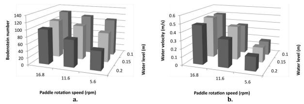
**Figure 8-1** Influence of paddle rotational speed, water level to Bodenstein number (a.) and water velocity (b.) in pilot HRAP.
