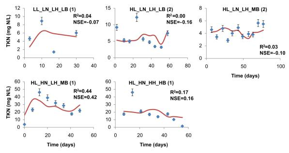
**Figure 10-3** Experimental TKN data at the effluent (diamond with error bars indicating measurement uncertainty) of different modalities (graph title with best fit order in brackets) fitted to the coupled RTD and mixed-order model (line).
