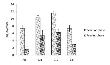
**Figure 7-2** Average with standard error of dissolved oxygen (DO) concentration in different test reactors during reaction phase and feeding phase.
