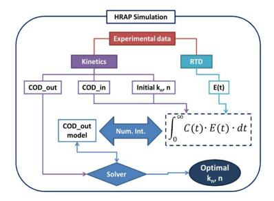
**Figure 6-1** General procedure of HRAP simulation.
