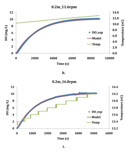
**Figure A 14** Fitting curves of each dynamic test for k<sub>L</sub>a determination.
