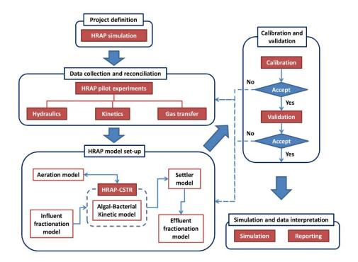
**Figure 11-1** General illustration of the HRAP simulation procedure.
