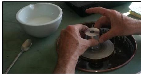
Figure 13: Polishing of the piezoelectric element.
