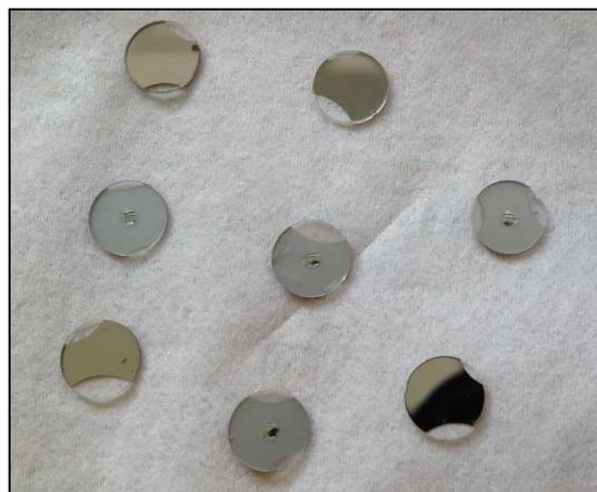
**Figure 26: Silica glass of the transducers with and without the lens**
