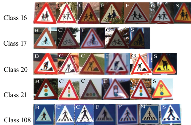
FIGURE 2.7 – Examples of some classes that contain intra class variability. Letters in the images are the initial of the country name they belong to. For example, B stands for Belgium, C for Croatia, etc.
