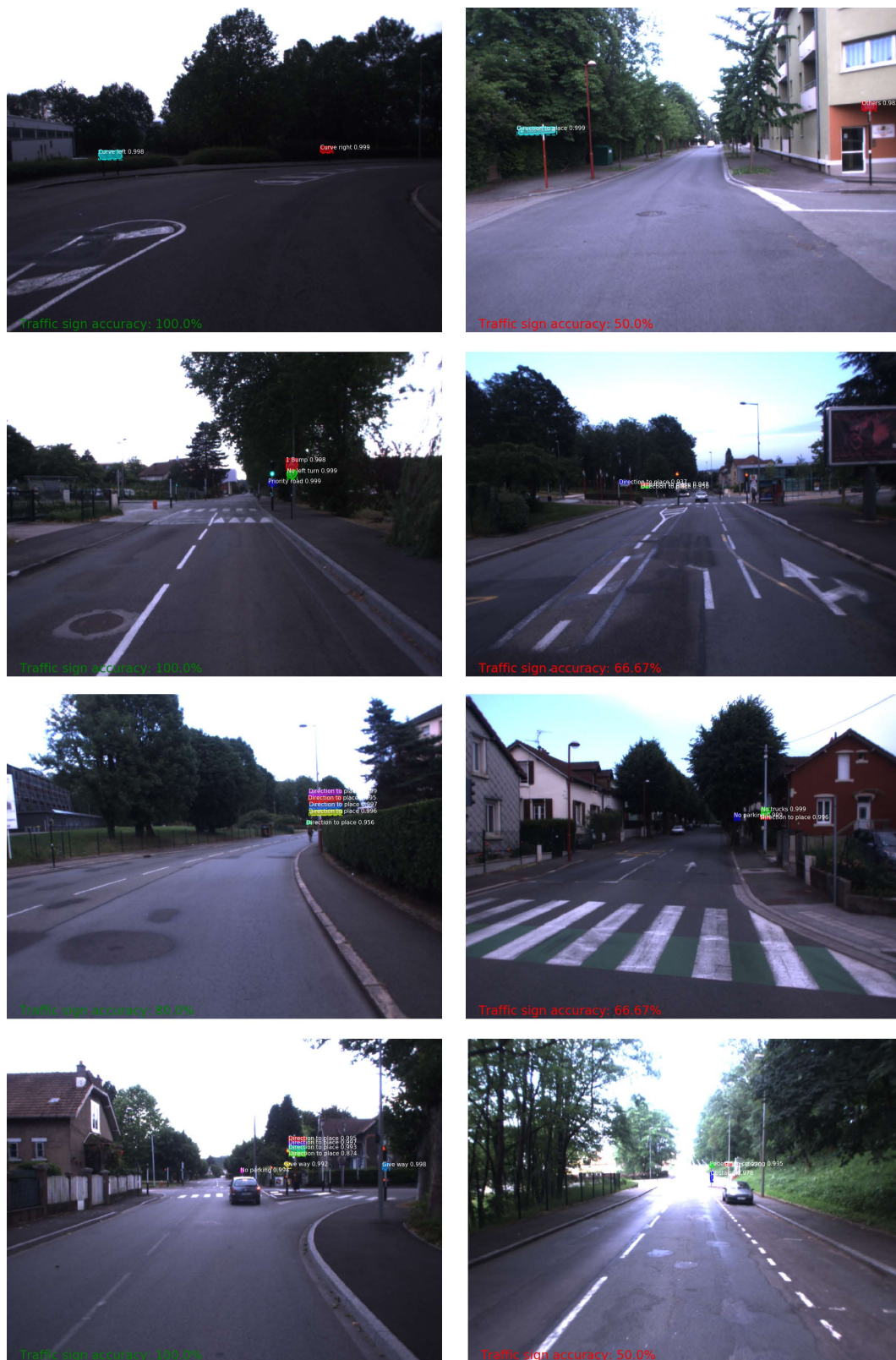
FIGURE 4.15 – Example of detection and classification results by our proposed traffic sign recognition module on UTBM-2 dataset. The recognition is performed with Mask R-CNN + Urban_Class_CNN trained in the urban set of the ETSD to detect 132 classes. The left column shows image examples with recognition accuracy above 75% while the right column shows images with traffic sign recognition accuracy under 75%.
