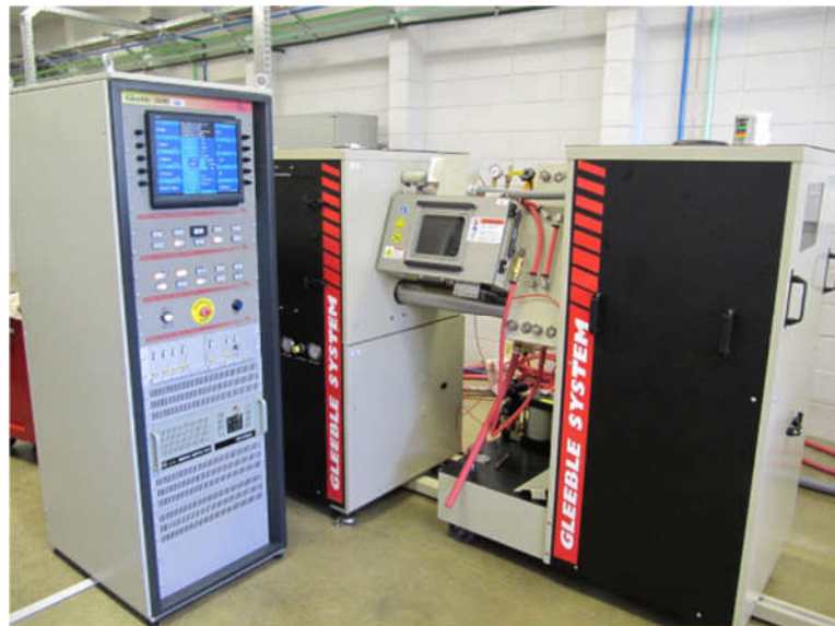
Figure 3-4: Gleeble 3800 MCU for tensile test – (LNLS- Brazil courtesy) 1
