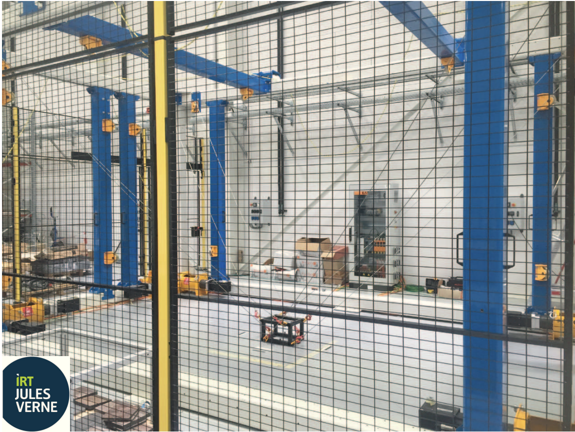
Figure I.12 – CAROCA prototype : a reconfigurable CDPR (Courtesy of IRT Jules Verne, Nantes)
