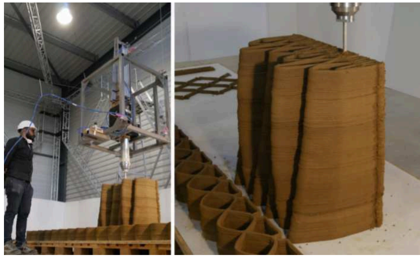
Figure I.8 – Cogiro, Pylos and the high print being processed [IDH + 18]
