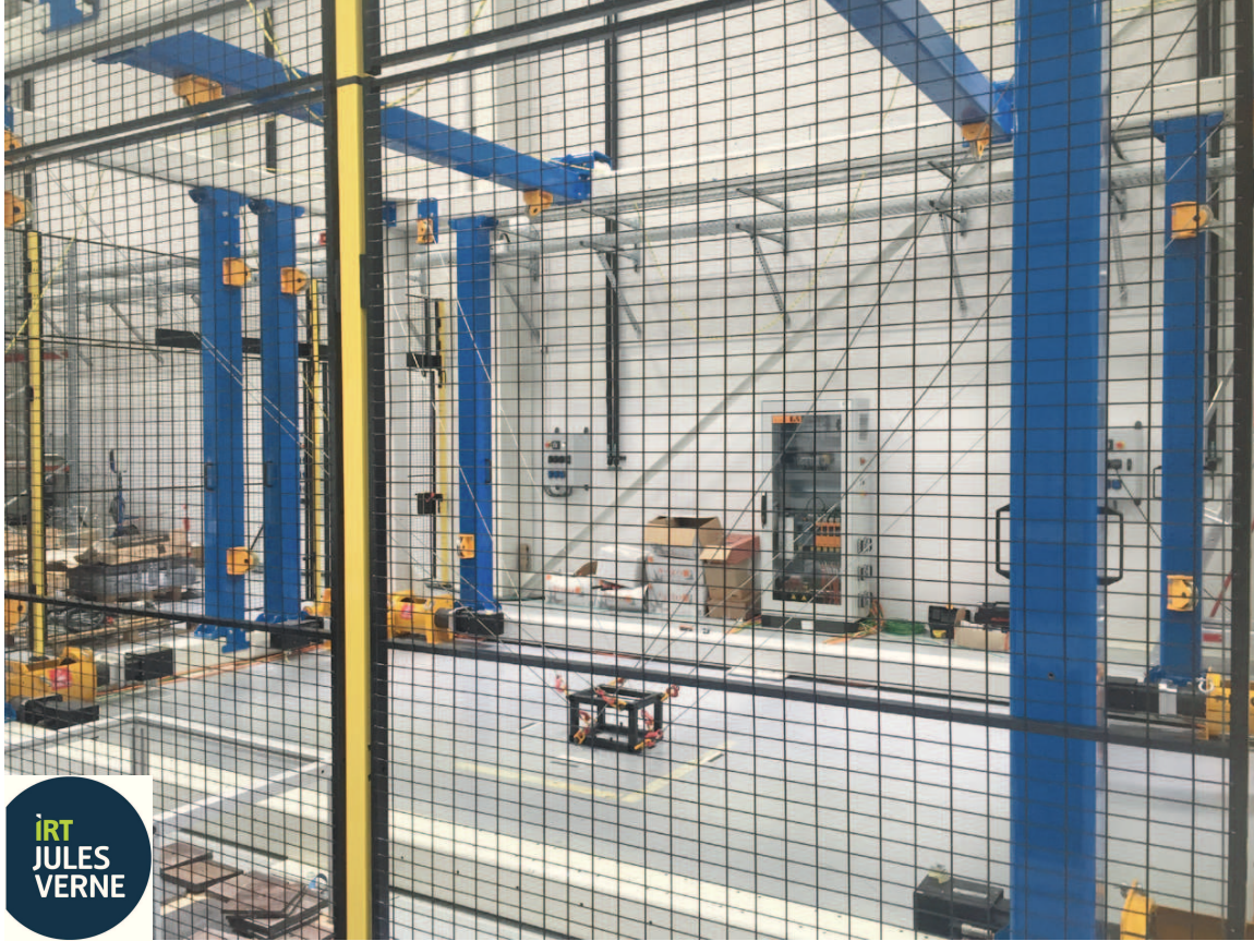
Figure 1.12 – CAROCA prototype : a reconfigurable CDPR (Courtesy of IRT Jules Verne, Nantes)
