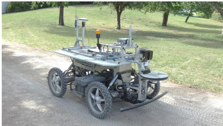
FIGURE A.1 – Robot mobile RobuFAST.
